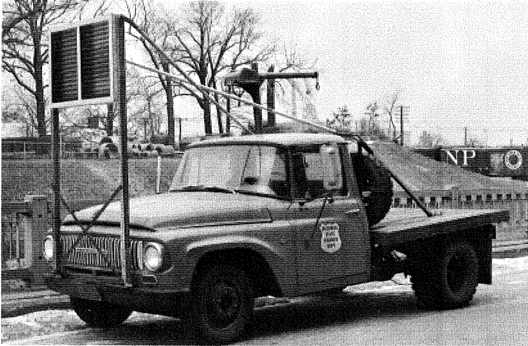
Figure 6. Truck-mounted louvered sign models for determining dynamic instability. Speed attained, 70 mph.
