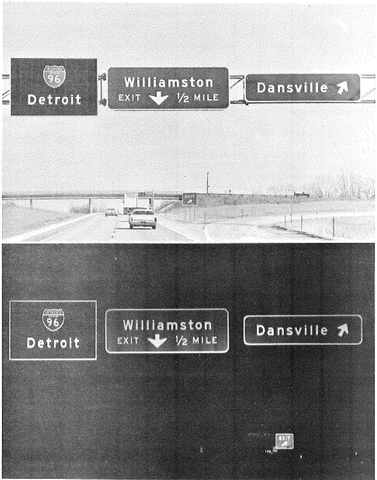
Figure 13. Mounted full-size louvered sign model showing night (a) and day (b) legend contrast.
