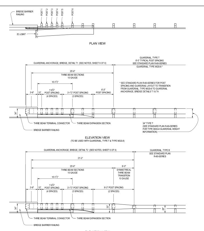
ELEVATION VIEW (TO BE USED WITH GUARDRAIL, TYPE B)
