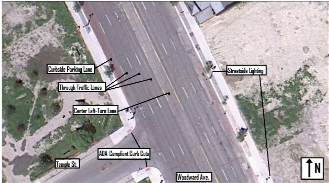
Figure 20. Aerial View of Woodward Avenue ROW
