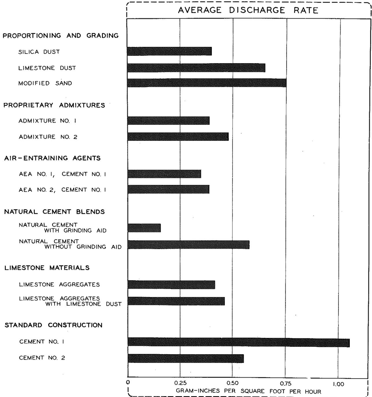
Figure 21. Rate of water passage through core sections.
