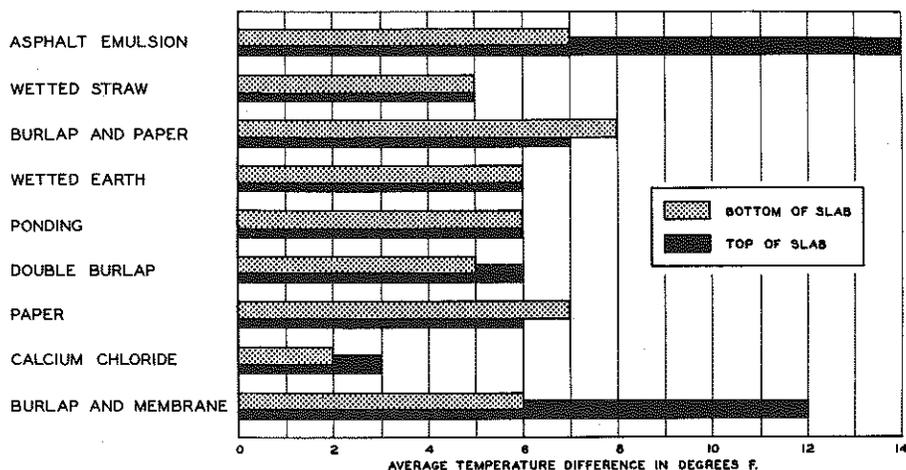
Figure 29. Average temperature difference between air and top and bottom of slab.
