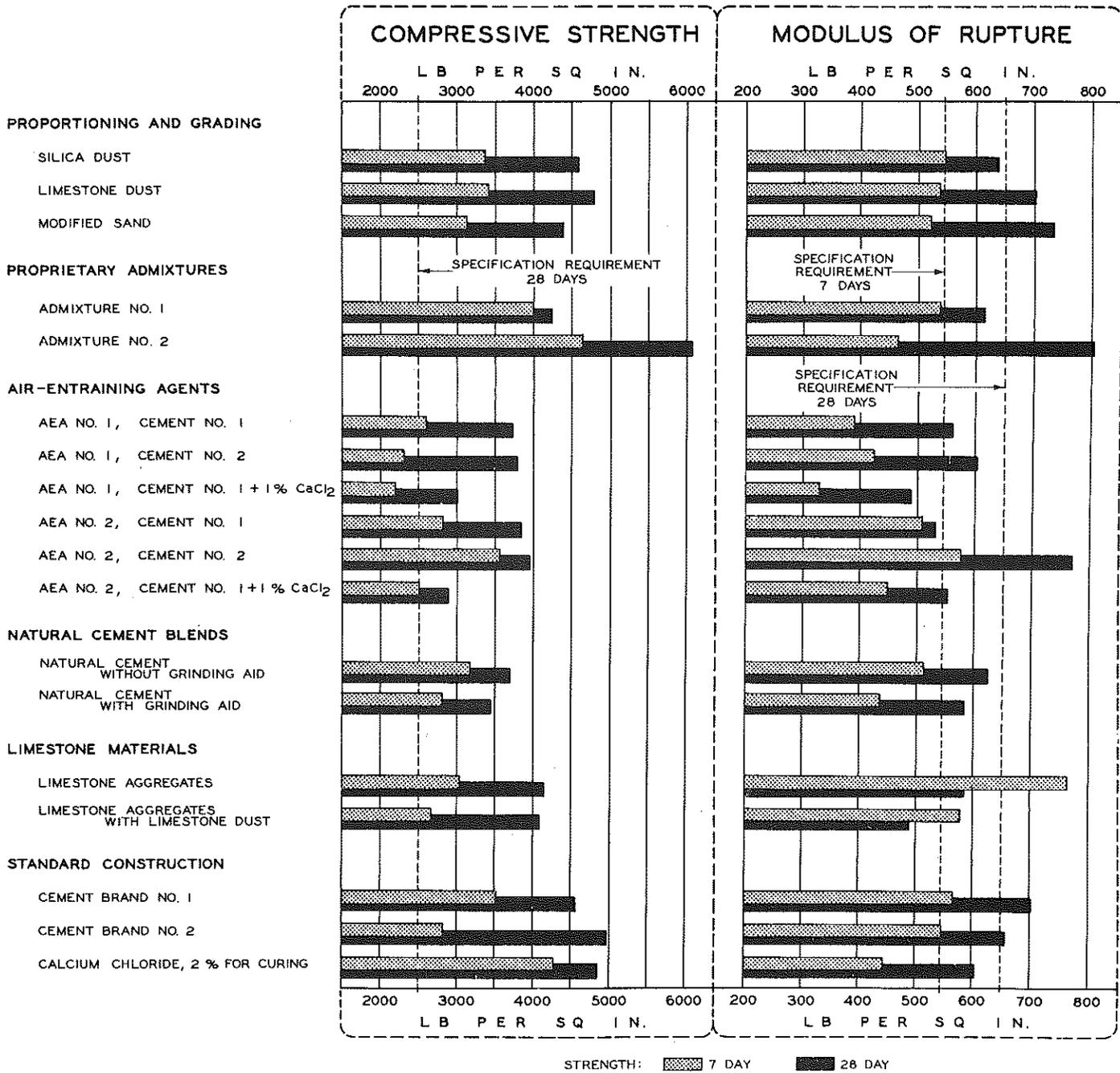
Figure 28. Compressive and flexural strengths of field-molded specimens.
