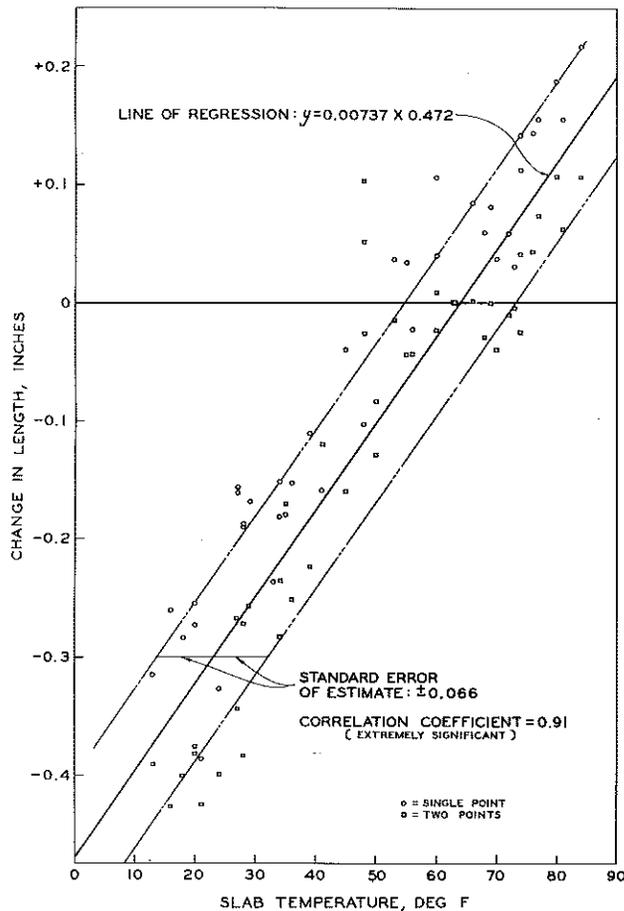
Figure 32. Change in 120-ft slab length with temperature for standard concrete with Cement No. 1.
