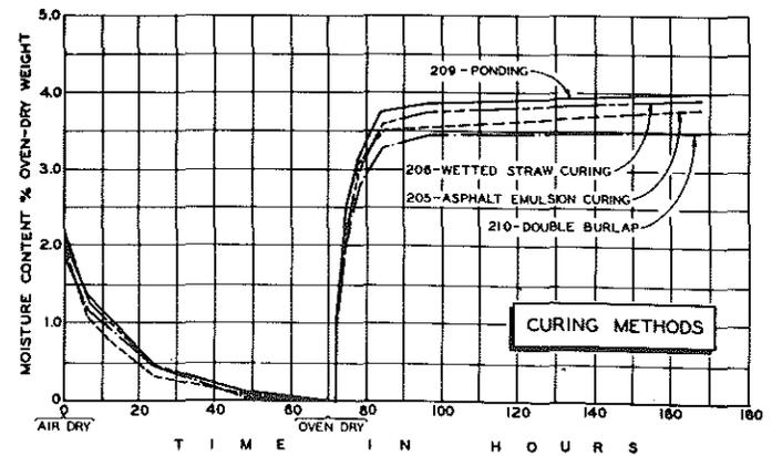
Figure 19. Rate of absorption of pavement cores.
