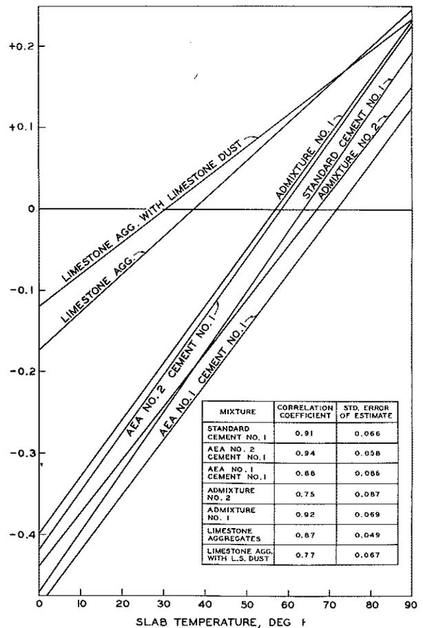
Figure 33. Comparison of slab length changes for seven concretes.
