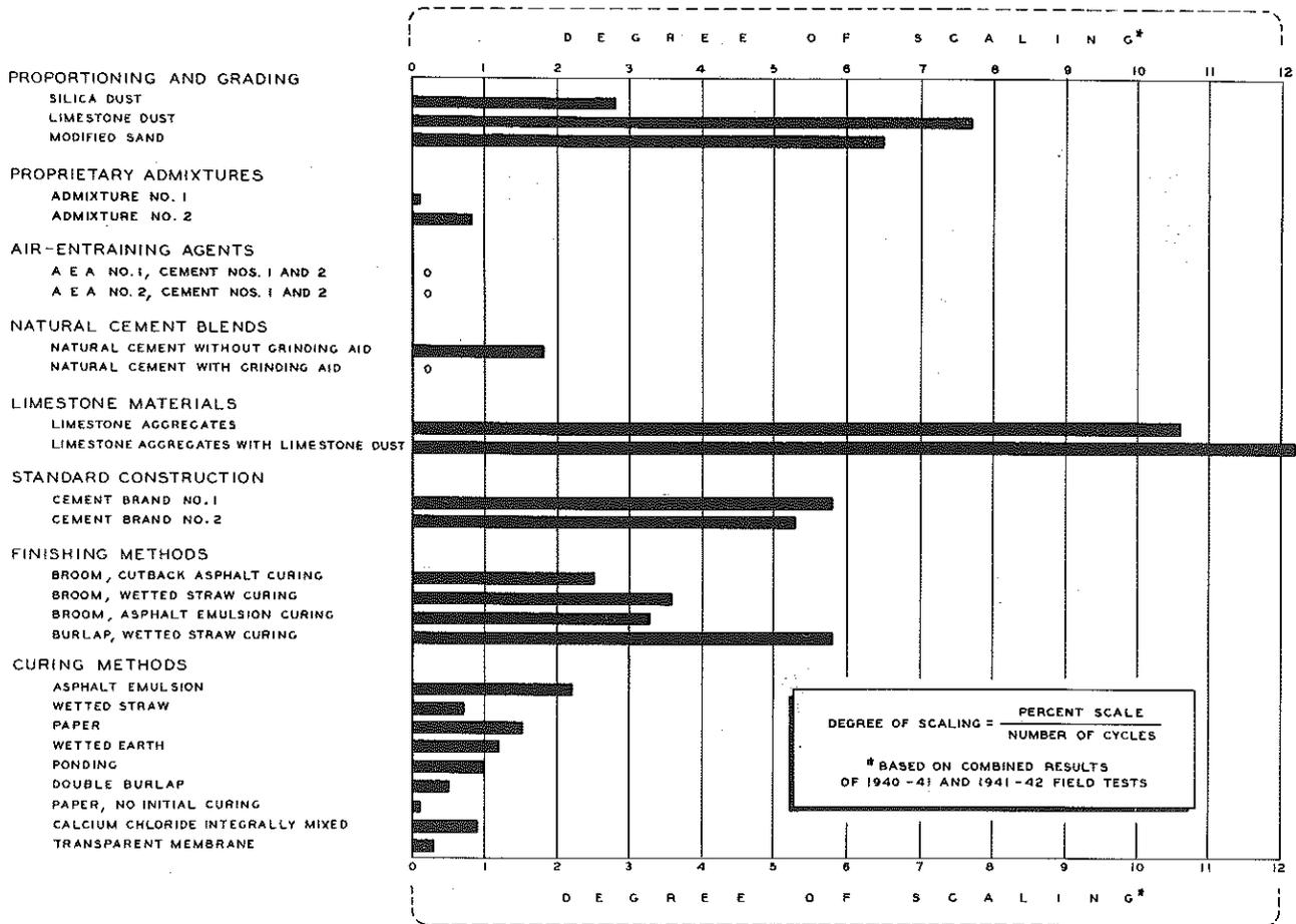
Figure 12. Scaling of experimental pavement sections in accelerated test.
