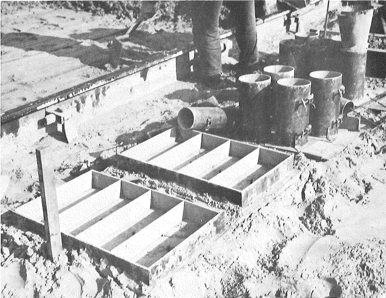
Figure 14. Steel molds ready for casting field specimens.
