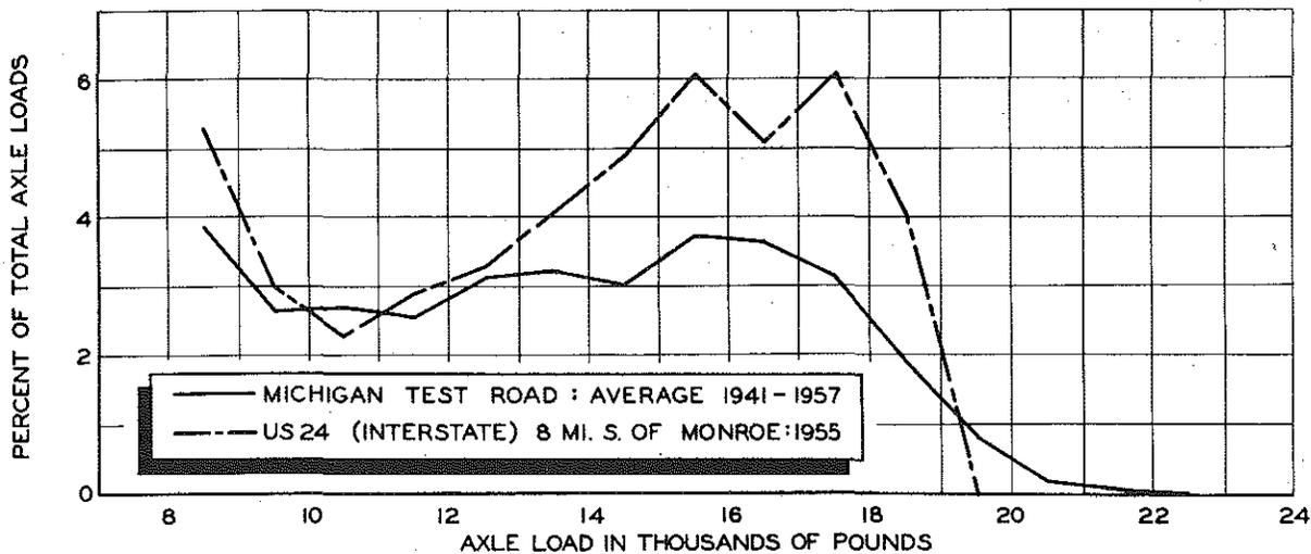
Figure 7. Axle load frequency.
