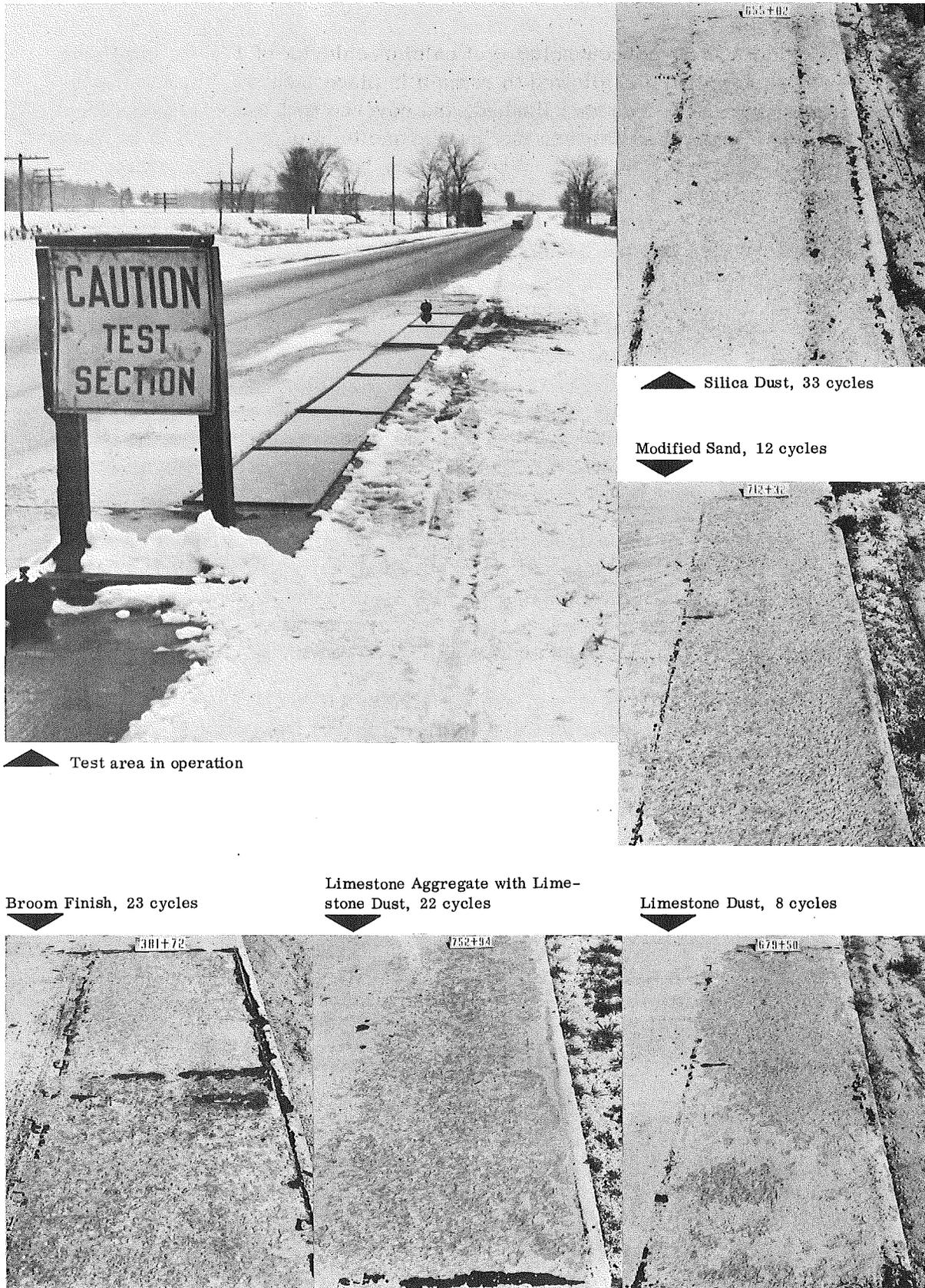
Figure 11. Condition of typical panels at end of accelerated scaling test.
