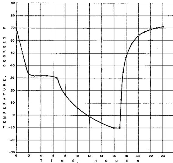
Figure 15. Freezing and thawing temperature cycle.
