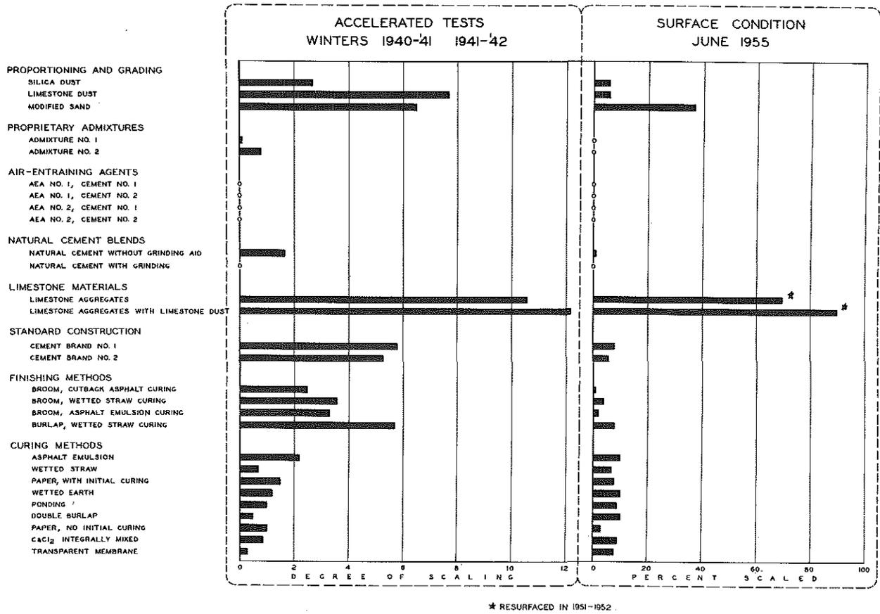
Figure 34. Comparison of accelerated sealing tests with pavement performance.
