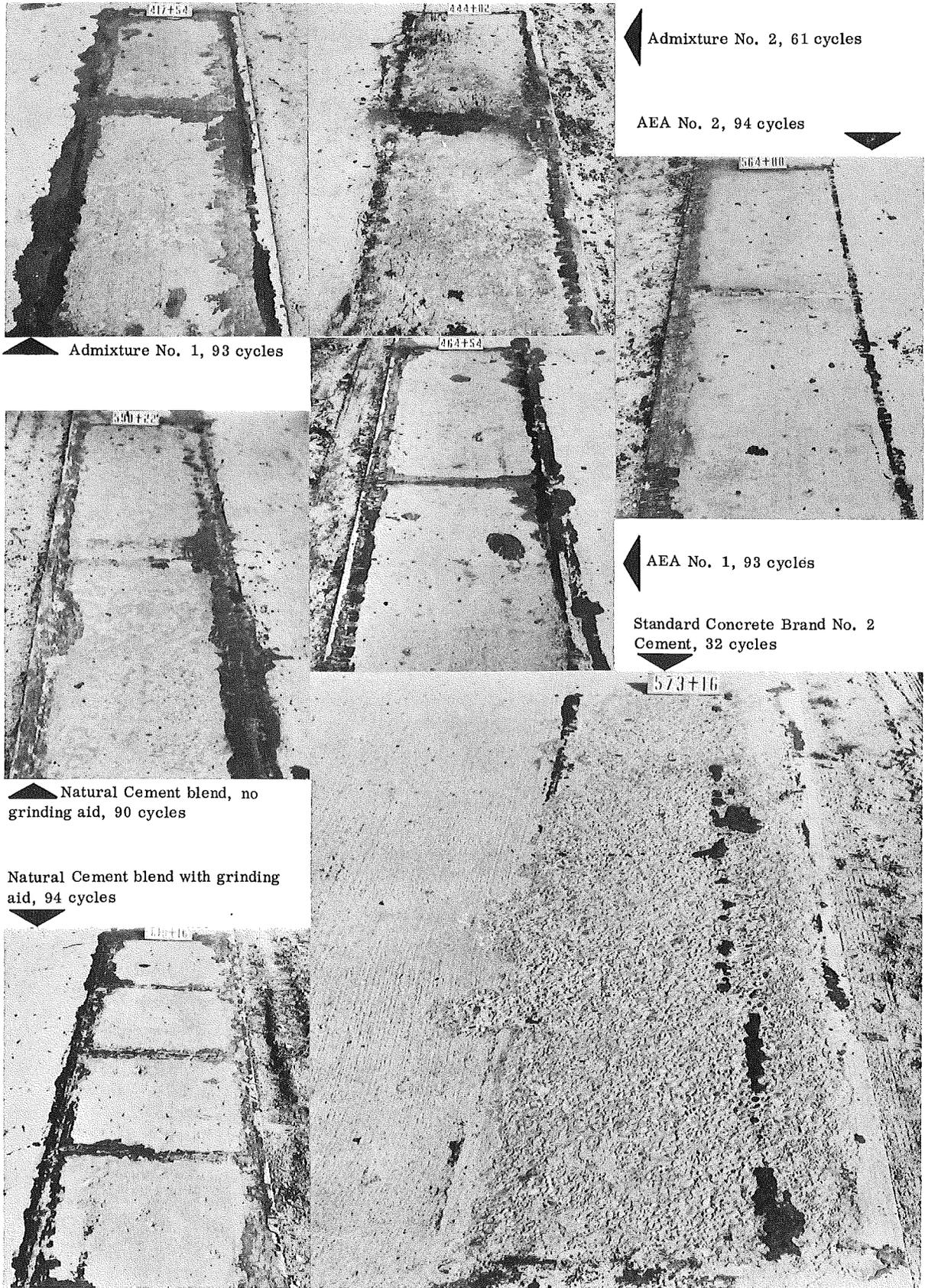
Figure 11. Condition of typical panels at end of accelerated scaling test (continued).
