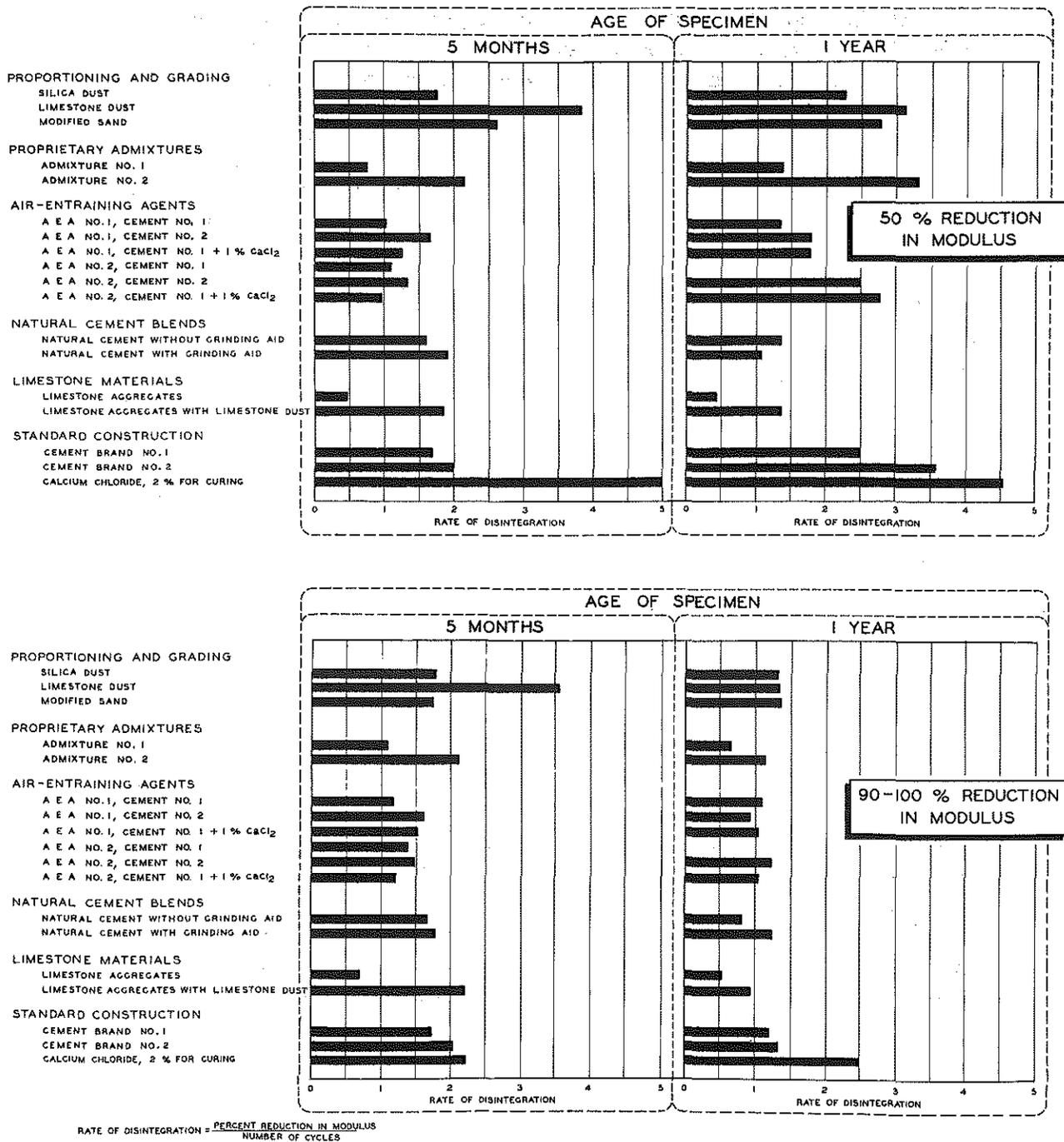
Figure 16. Rate of disintegration of field molded specimens by freezing and thawing in water.
