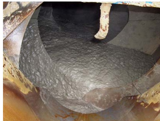
Figure 4.13. ECC Material in Mixer
