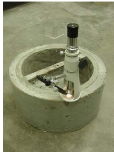
Figure 6.24. Restrained shrinkage ring test with crack width measurement microscope.
