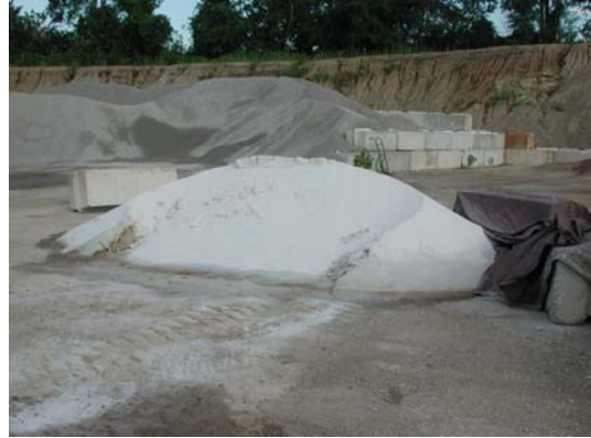
Figure 5.5. F-110 Silica Sand batching pile outside Clawson Concrete
