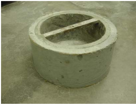
Figure 6.23. Restrained shrinkage ring test.
