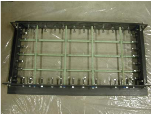
Figure 6.26. Top view of large restrained shrinkage test setup
