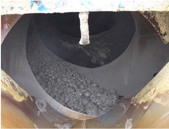
Figure 4.11a. Cement Balls Formed During Mixing.
