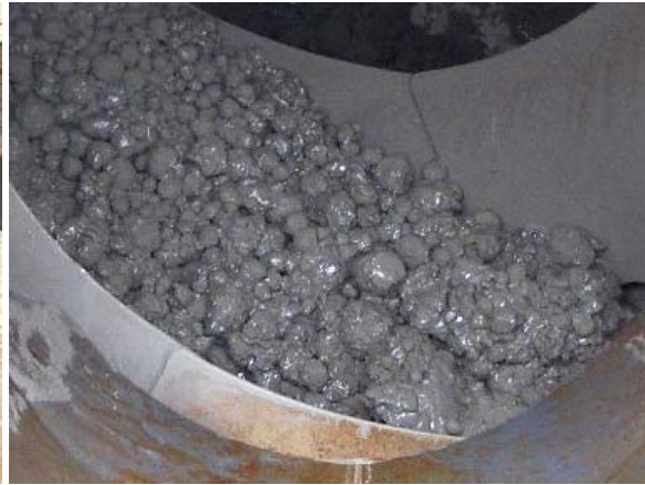
Figure 4.11b. Close-up view of Cement Balls Formed During Mixing
