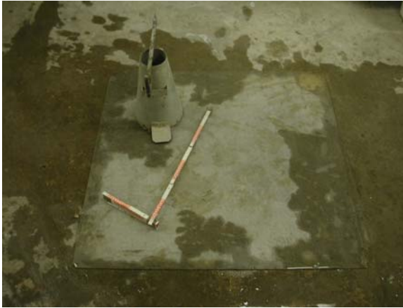
Figure 4.3a. Deformability test setup
