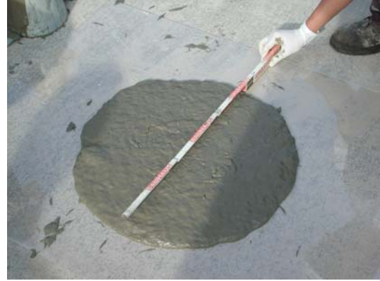
Figure 5.9. Slump cone measurement.
