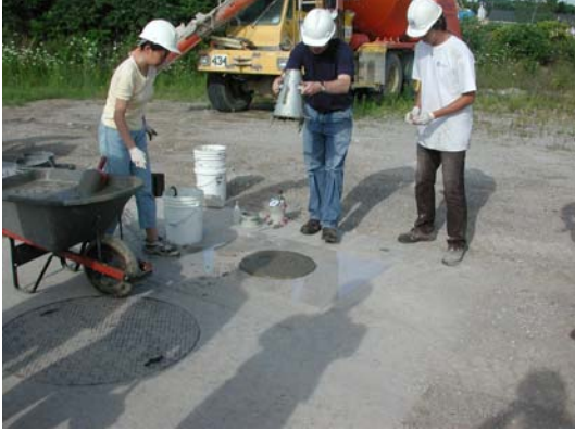
Figure 5.8. Slump cone testing.
