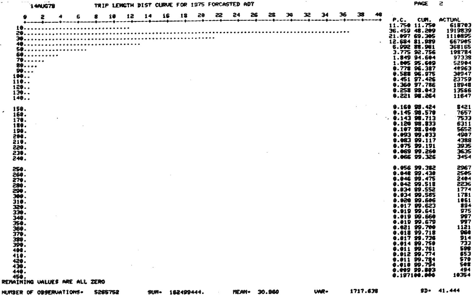
sometimes not taken on the most local traveled roads since they are the most difficult to survey due to traffic congestion. The conclusion then in reviewing these TLD curves is that the model is doing an excellent job of matching the actual travel based on the number of trips generated and distributed by trip length class. This does not mean, however, that these trips are utilizing the right roads, which brings us to the next step.
