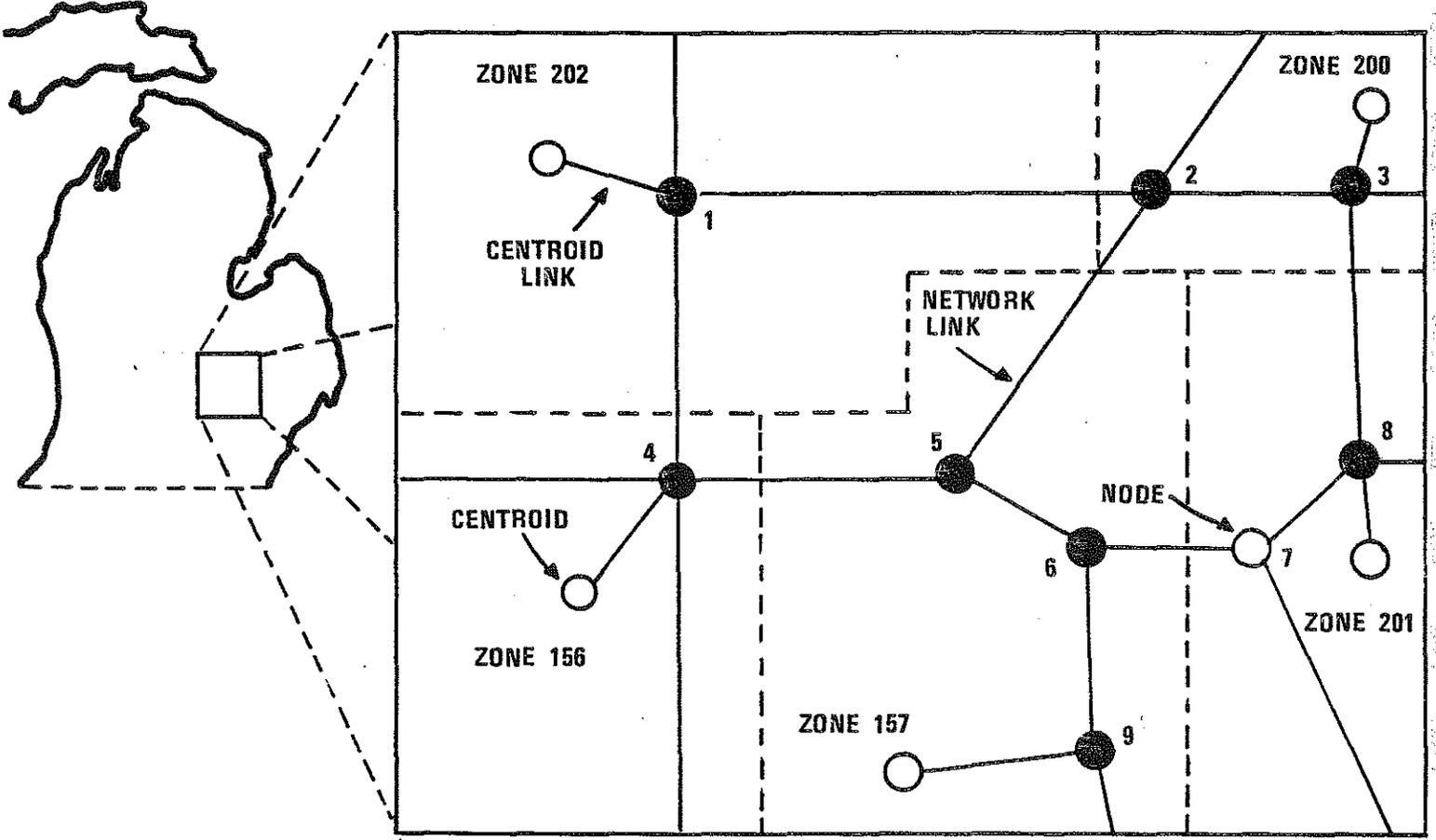
includes information such as speed, distance, and capacity information. Since the 1975 network was created through standard coding procedures, this same technique can be used to simulate alternate highway proposals. The output from the network portion of the modeling system is a primary part of the travel forecasting process.
