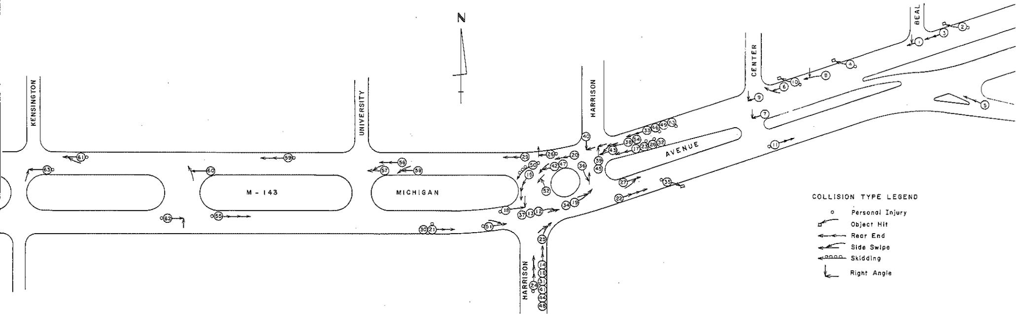
FIGURE 2: COLLISION DIAGRAM ONE YEAR BEFORE CONSTRUCTION - 9-1-73 Through 8-31-74.
