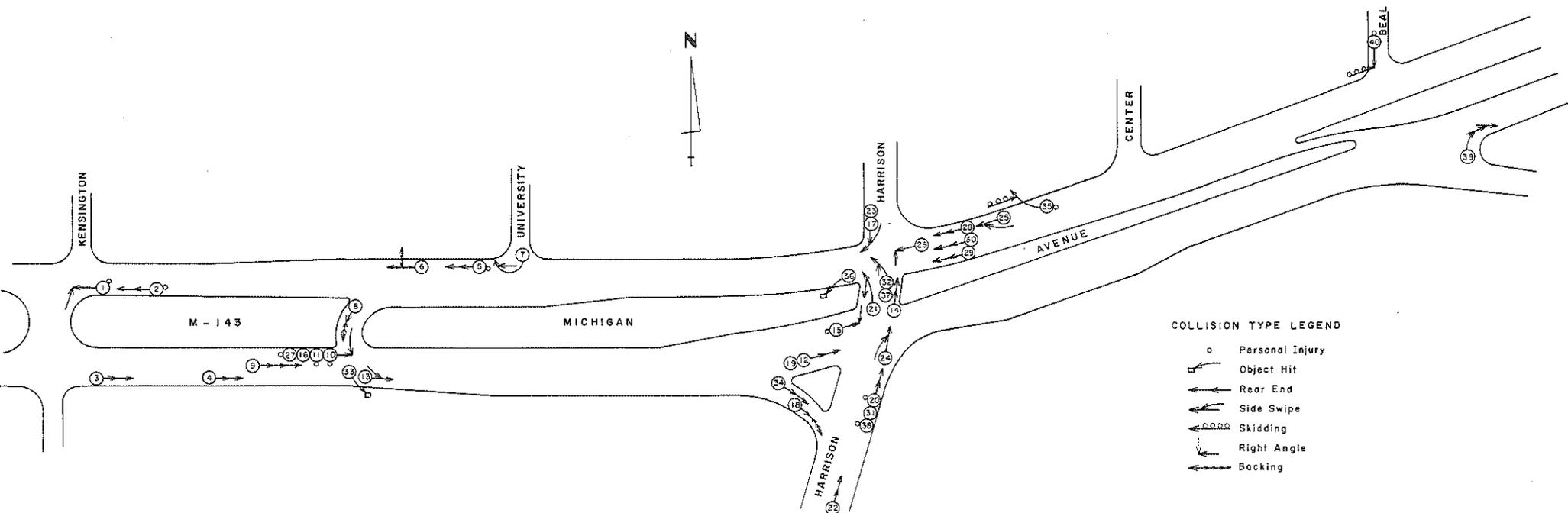
FIGURE 3: COLLISION DIAGRAM ONE YEAR AFTER CONSTRUCTION - 12-1-74 Through 11-30-75.
