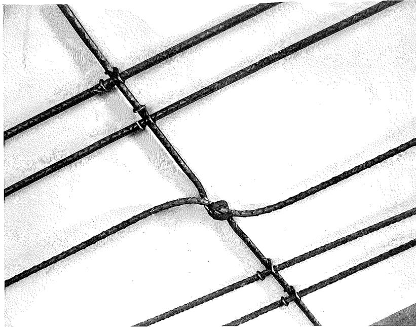
Figure 10. Distortion of hinge under tension.
