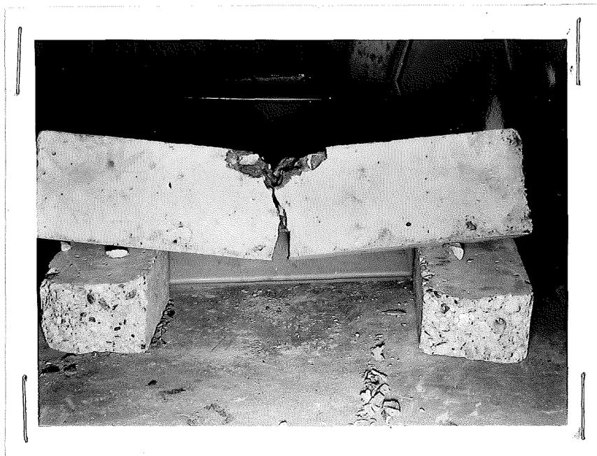
Figure 16. Specimen with continuous bar. Concrete failed in compression. Bar still unbroken.
