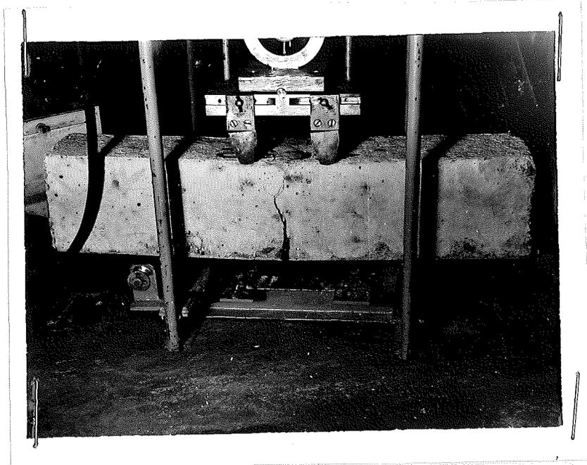
Figure 15. Failure of concrete specimen containing continuous bar
