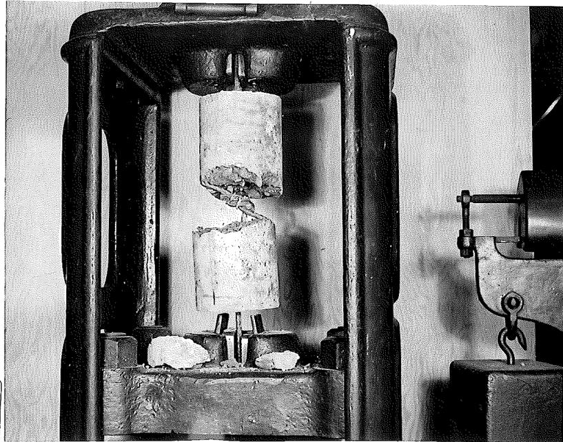
Figure 12. Typical failure of hinge.
