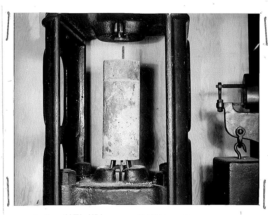
Figure 13. Bond test of lapped bars.
