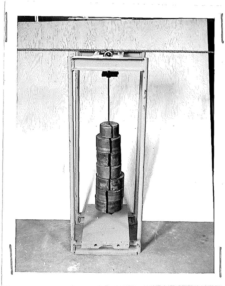
Figure 7. Method of testing clip under tension.
