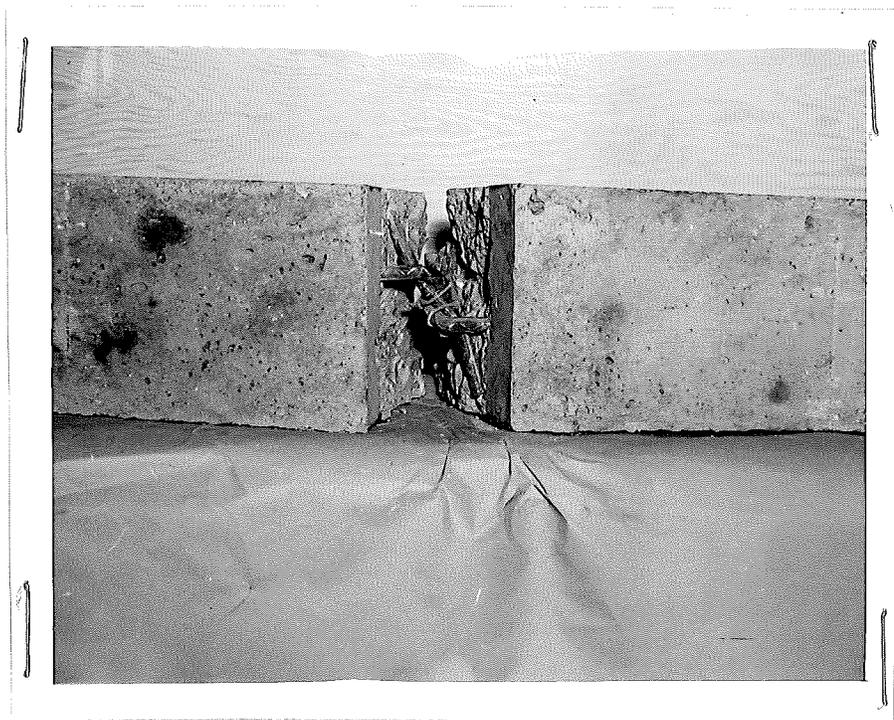
Figure 14. Failure of hinge in modulus of rupture test.
