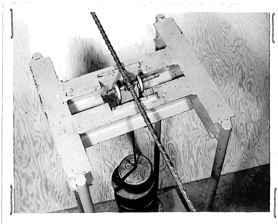
Figure 8. Close view of clip under tension.
