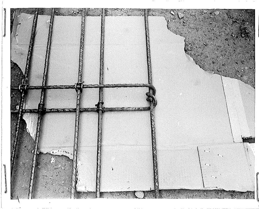
Figure 5. View of hinge in folded position.
