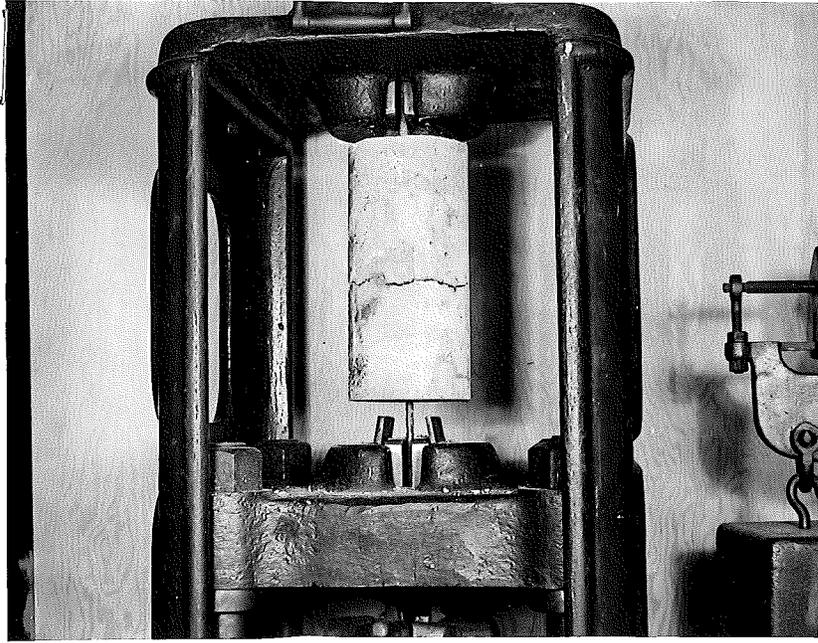
Figure 11. Cracking of concrete specimen containing hinge.
