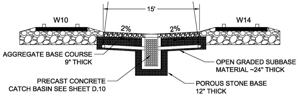
**Figure 3-4: Proposed Drainage Detail**
