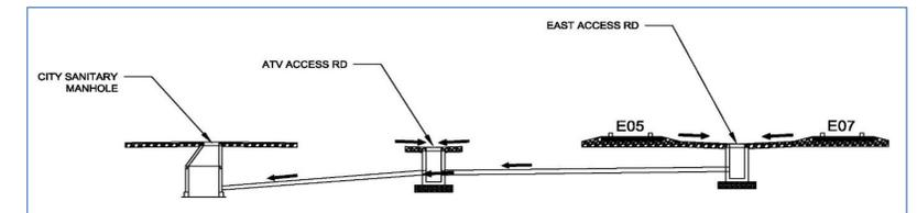
General Cross Section of Drainage Pipe in East Yard
