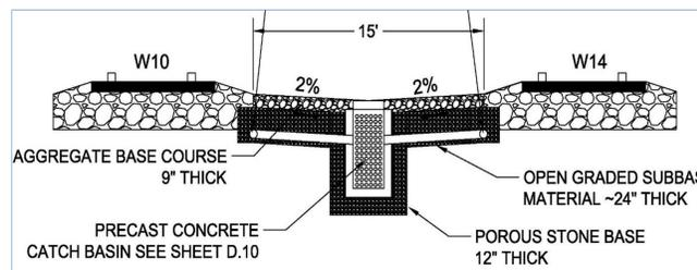
Detailed Catch Basin Cross Section With Underdrain
