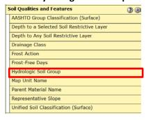
Select "View Rating" and be sure there is a check next to "Table" in order to obtain a table of Hydrologic Soil Group (Rating Column) for each selected Soil Map Unit. If "Description of Rating" or "View Description" is selected, a description will be given of the hydrologic soil group ratings (Classes).
