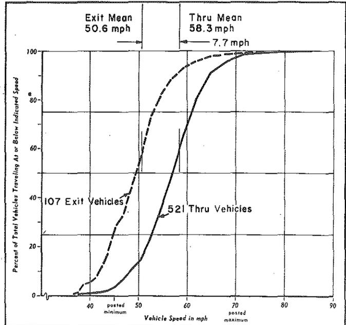
FIGURE 7. Thru and Exit Speeds US-27 @ Mannsiding Rd. (Enoscope Data)
