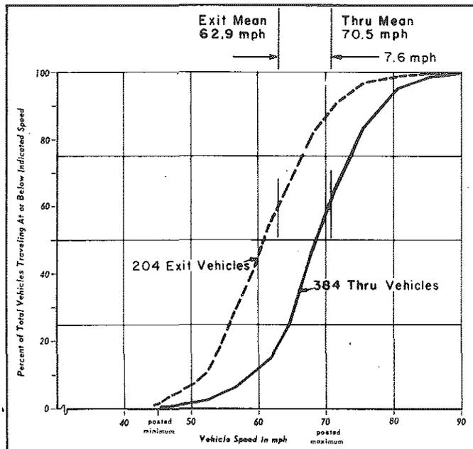
FIGURE 4. Thru and Exit Speeds
