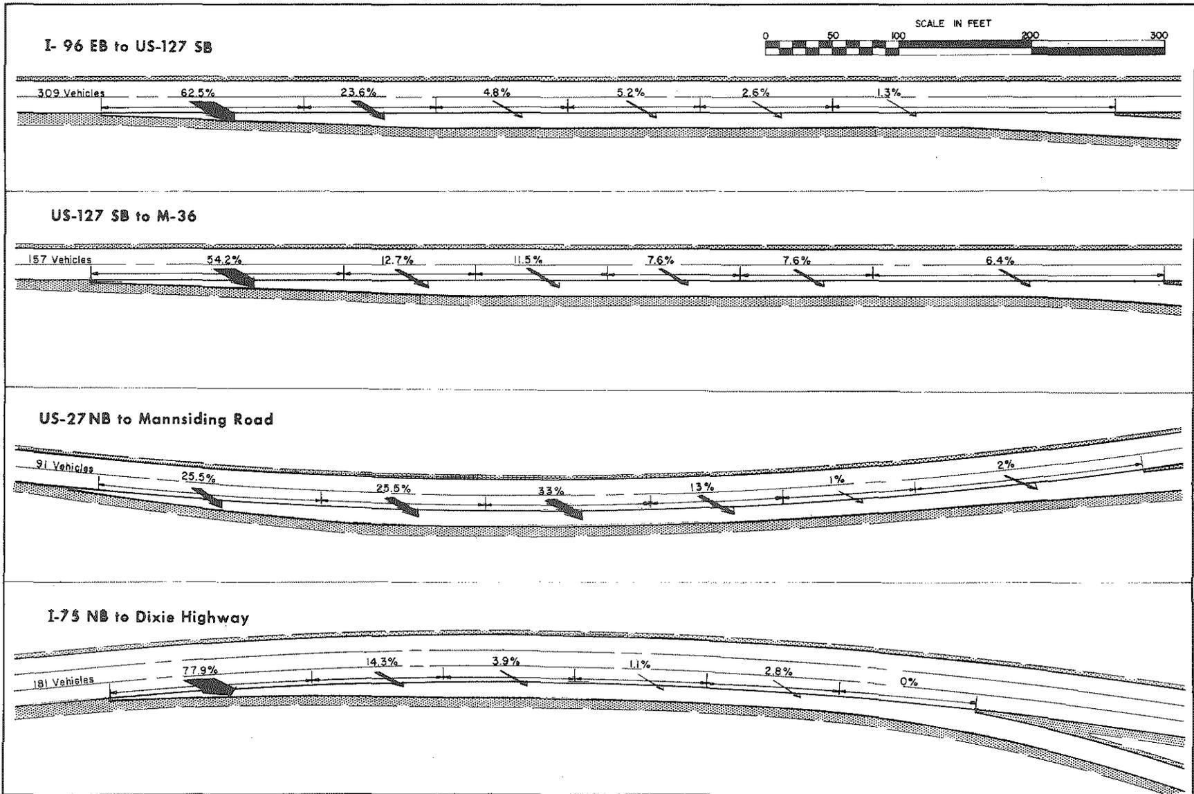
FIGURE 15. Distribution of Entry Zone Data, Parallel Ramps
