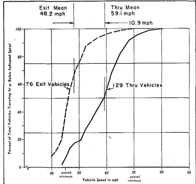
FIGURE 14. Thru and Exit Speeds I-96 @ Wixom Rd. (Enoscope Data)
