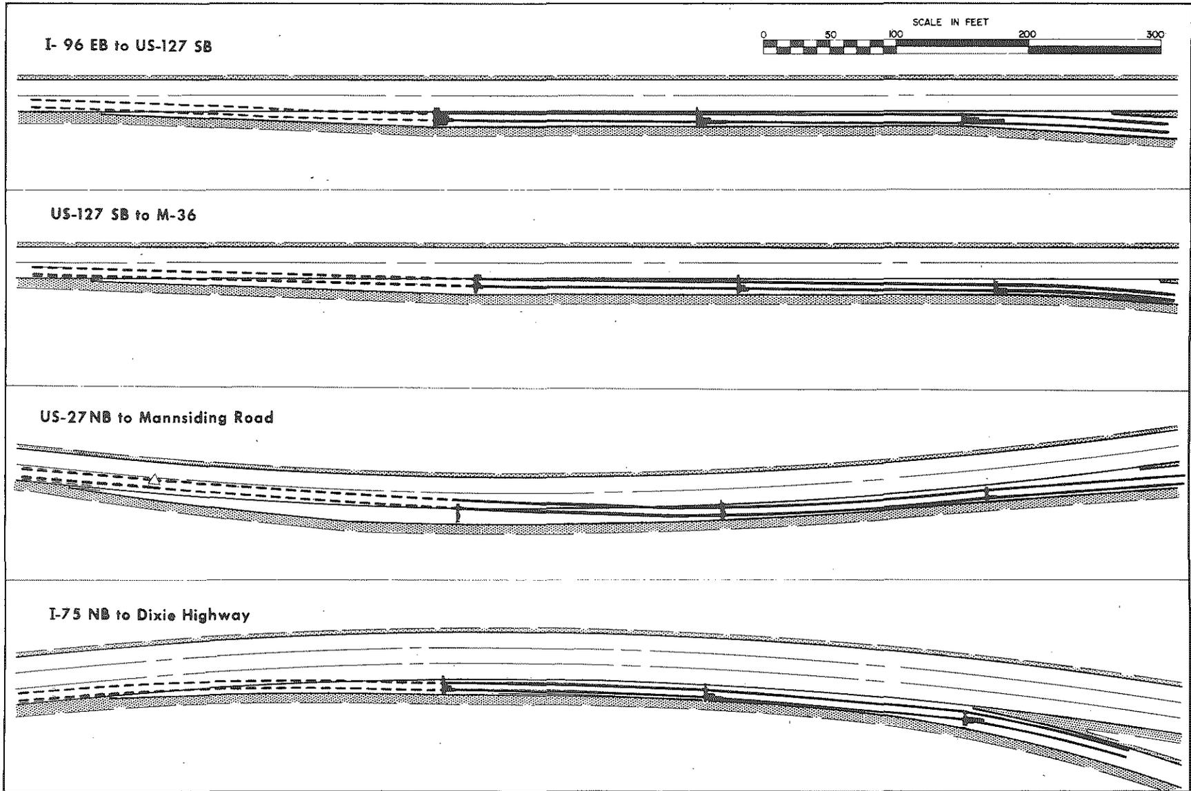
FIGURE 16. Distribution of Wheel Paths and Typical Paths, Parallel Ramps
