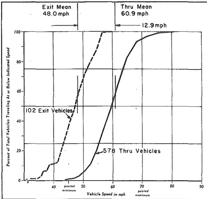
FIGURE 12. Thru and Exit Speeds
