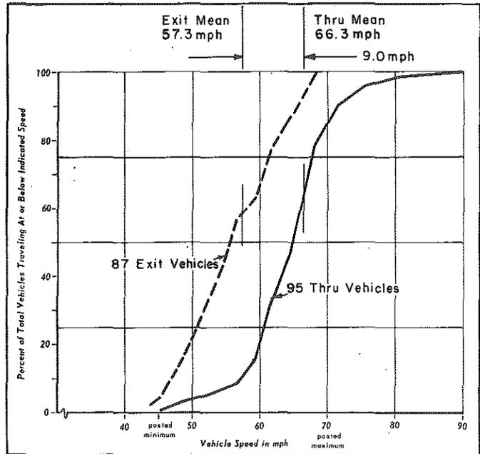
FIGURE 10. Thru and Exit Speeds I-496 @ I-96 (Enoscope Data)
