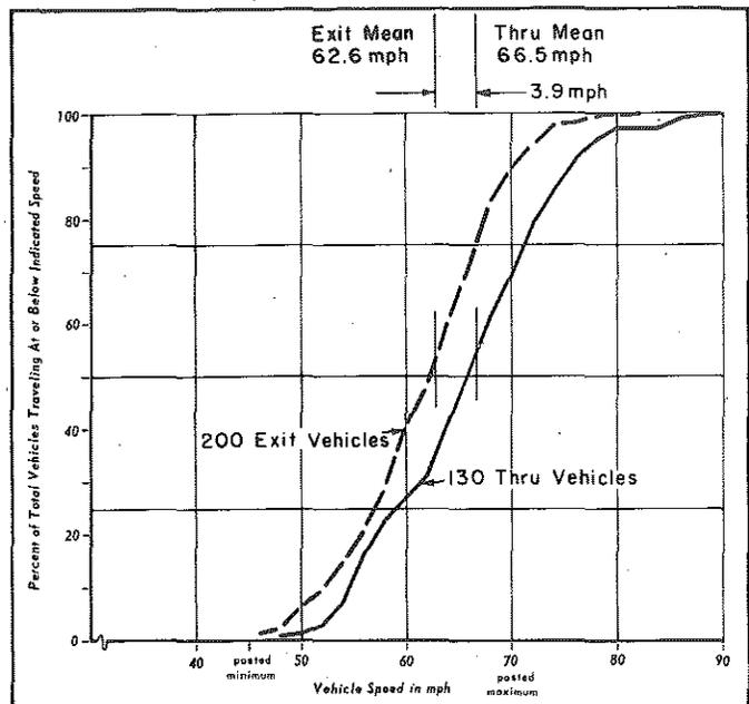
FIGURE 11. Thru and Exit Speeds I-496 @ I-96 (Electronic Data)
