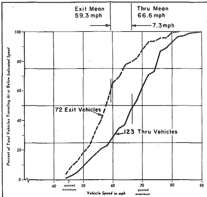
FIGURE 13. Thru and Exit Speeds
