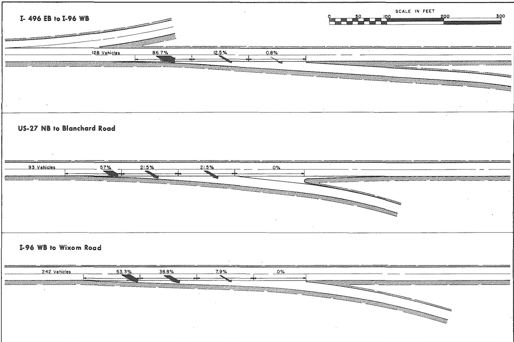
FIGURE 17. Distribution of Entry Zone Data, Taper Ramps
