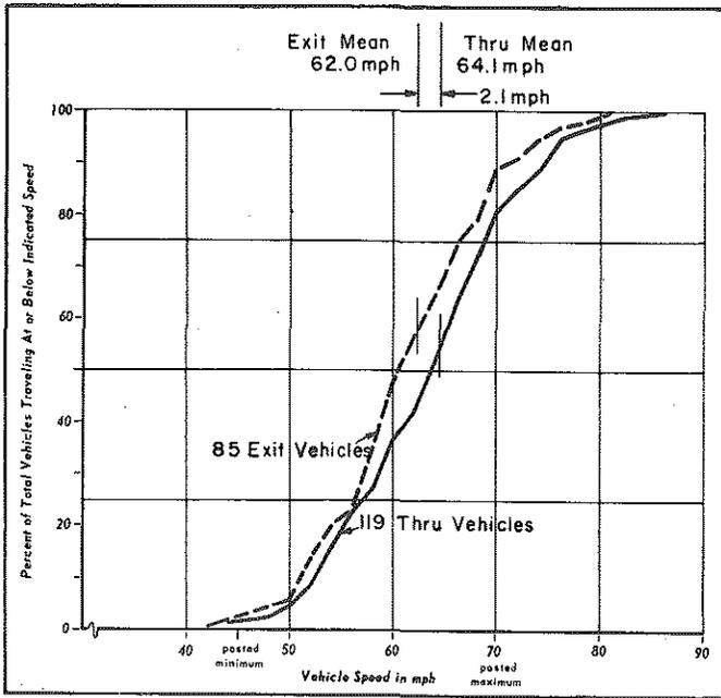
FIGURE 9. Thru and Exit Speeds I-75 @ Dixie Highway (Electronic Data)
