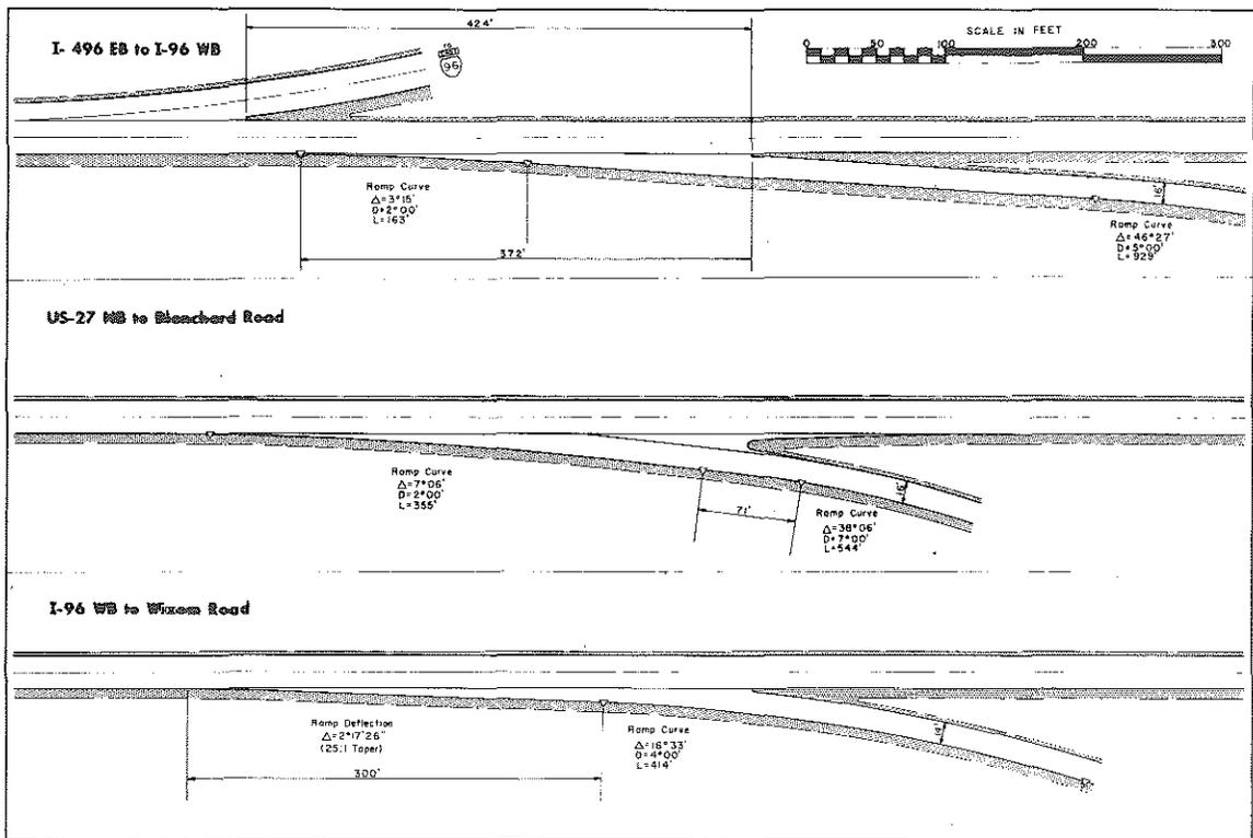
FIGURE 3. Horizontal Alignment of Taper Ramps
