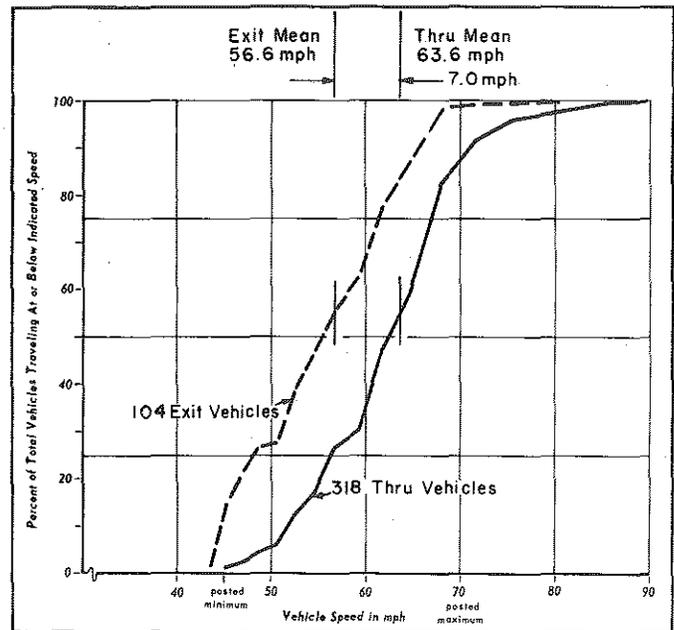
FIGURE 8. Thru and Exit Speeds I-75 @ Dixie Highway (Enoscope Data)
