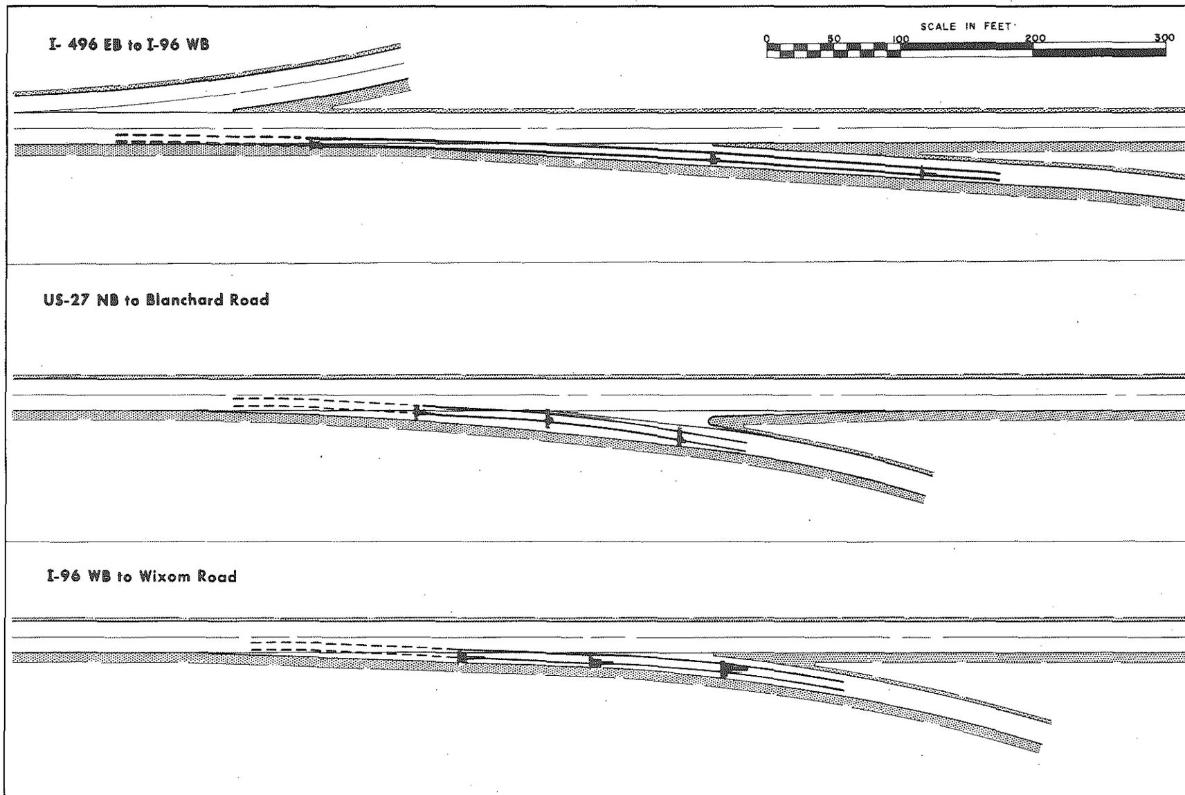
FIGURE 18. Distribution of Wheel Paths and Typical Paths, Taper Ramps
