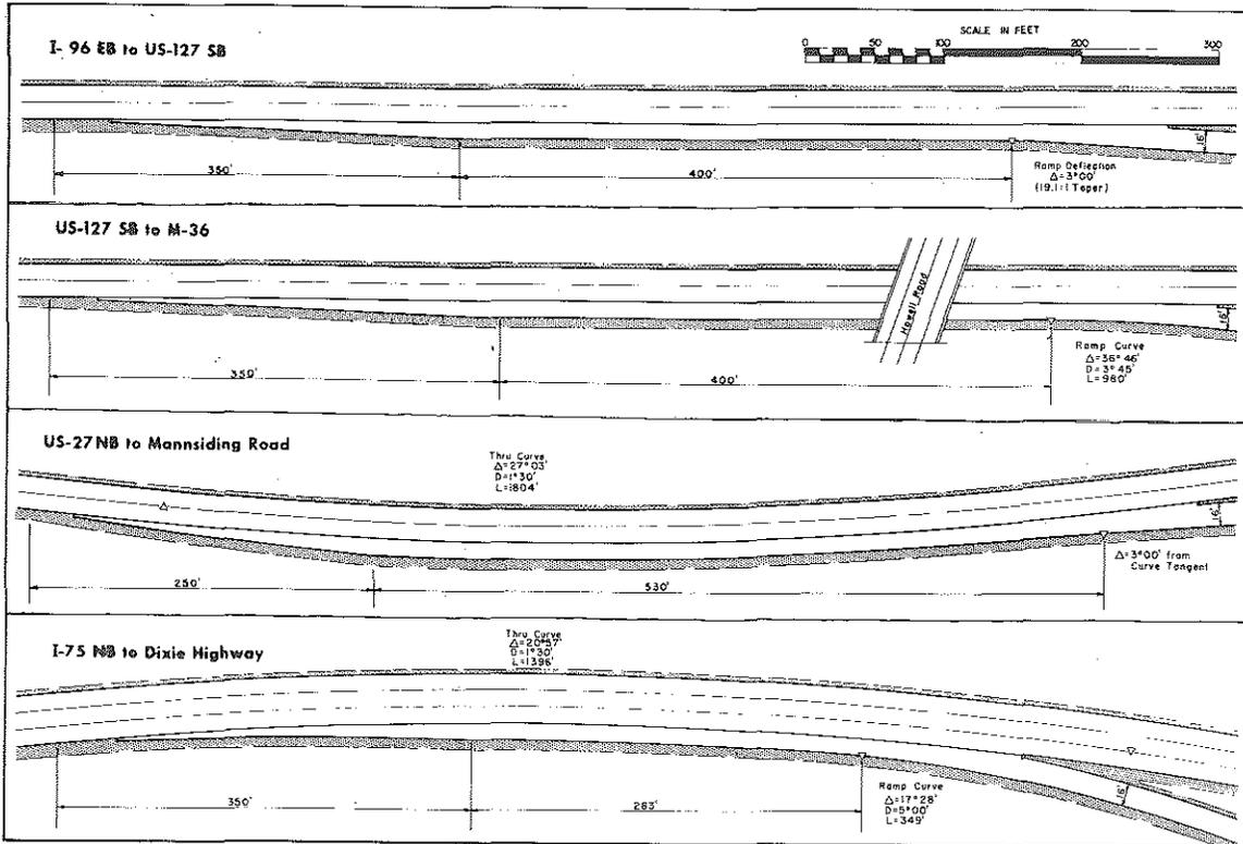
FIGURE 2. Horizontal Alignment of Parallel Ramps
