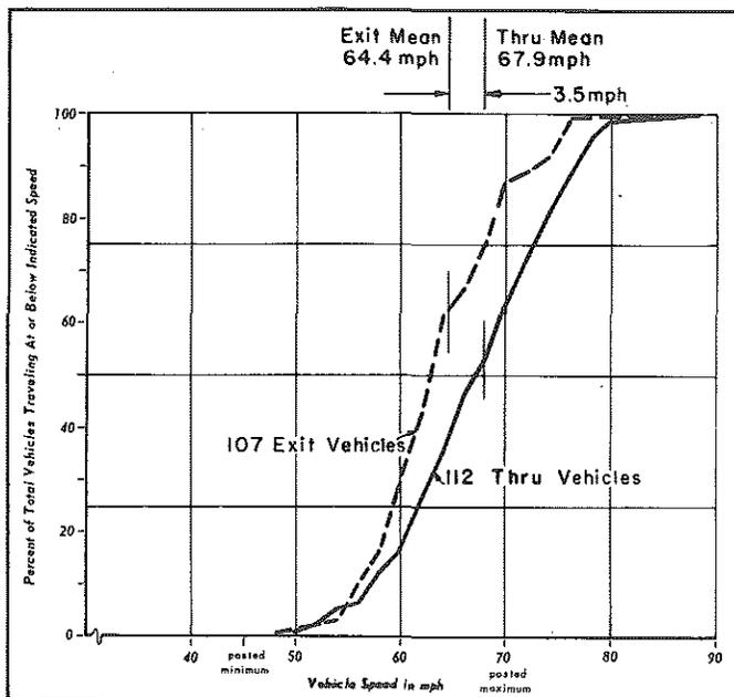
FIGURE 6. Thru and Exit Speeds US-127 @ M-36, (Electronic Data)
