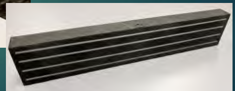
Section of Elastomeric showing steel shims
