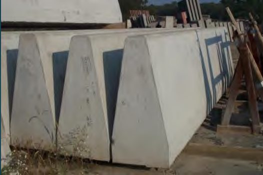
Single Slope Barrier
