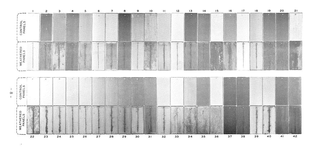
Figure 2. Series 3 panels with unexposed control panel above in each pair, and test-weathered panel with vertical scratch below (identification and performance ratings in Table 2).
