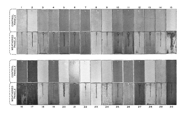
Figure 1. Series 2 panels with unexposed control panel above in each pair, and test-weathered panel with vertical scratch below (identification and performance ratings in Table 1).
