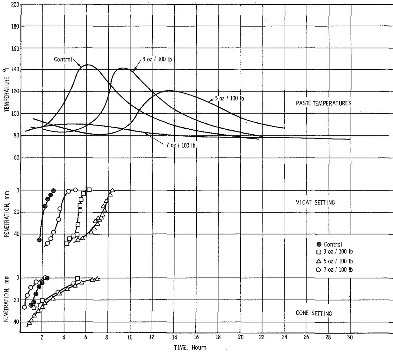
Figure 5. Same type of data as Figure 4—abnormal behavior (cement No. 1, admixture No. 1, 90°F).
