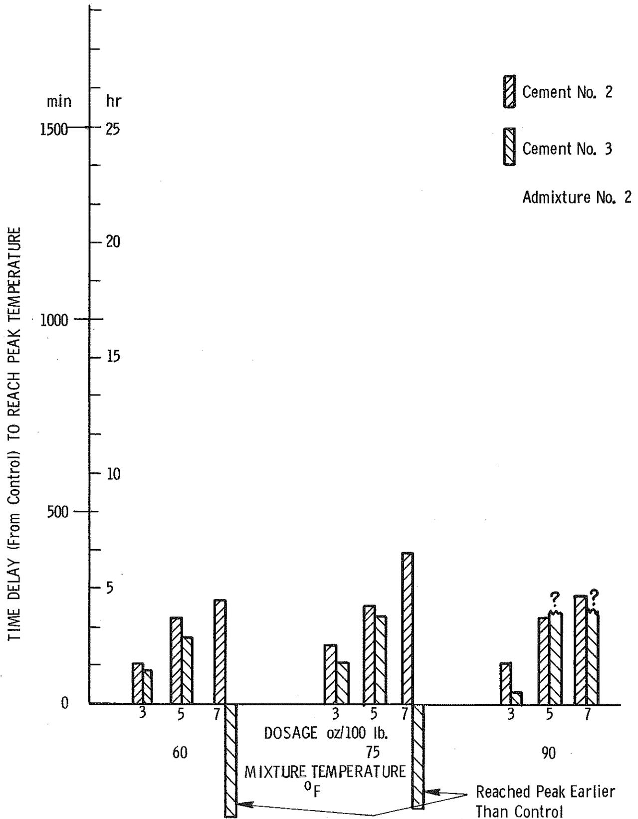
Figure 12. Delay from control in reaching peak temperature of pastes made with admixture No. 2.
