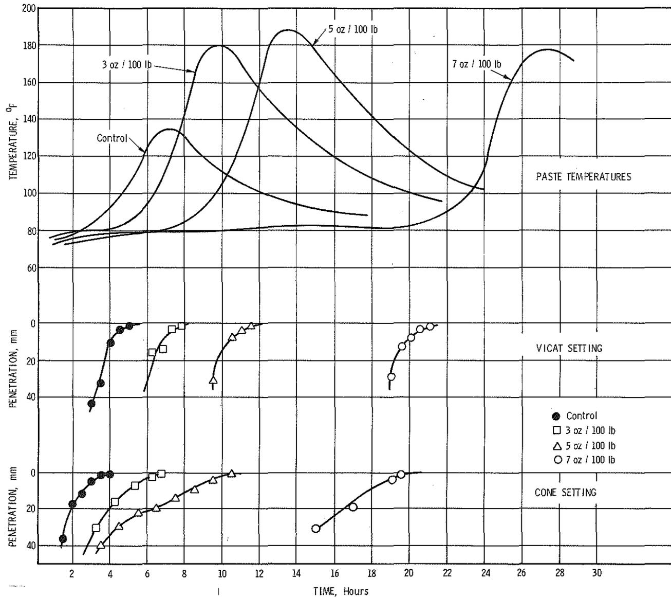
Figure 4. Adiabatic temperature rise and corresponding Vicat and cone setting of cement paste without admixture and at three dosages—normal behavior (cement No. 3, admixture No. 3, 75°F).
