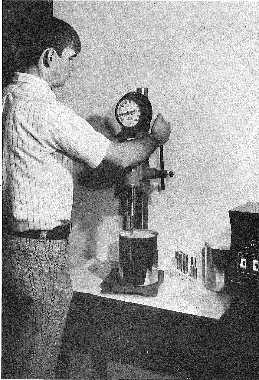
Figure 3. Apparatus used for time of setting of concrete by penetration resistance of sieved mortar.
