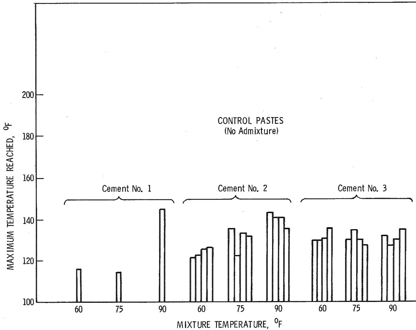
Figure 8. Maximum temperature attained in vacuum flasks—control pastes without admixture. Four repeat tests at each mixing temperature for cements Nos. 2 and 3.
