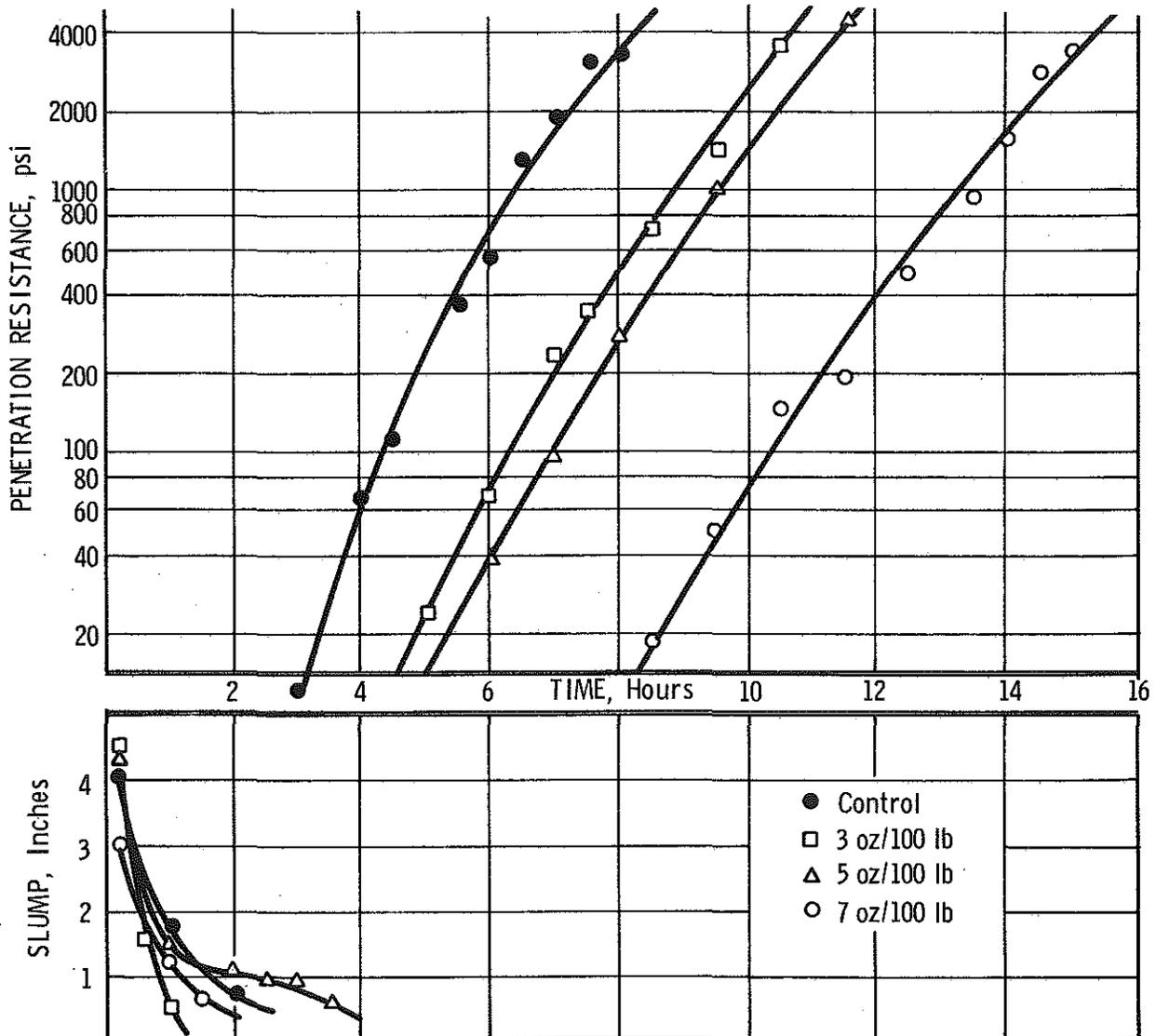
Figure 6. Penetration resistance and slump of concrete vs. time after mixing (cement No. 3, admixture No. 4, 60°F).
