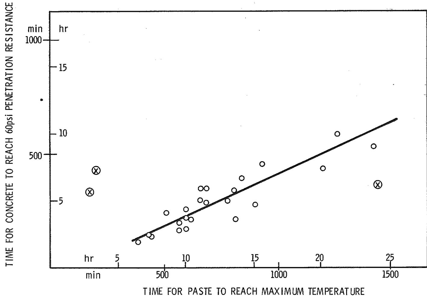
Figure 15. Time for concrete to reach 60 psi penetration resistance vs. time for paste to reach maximum temperature in vacuum flasks.
