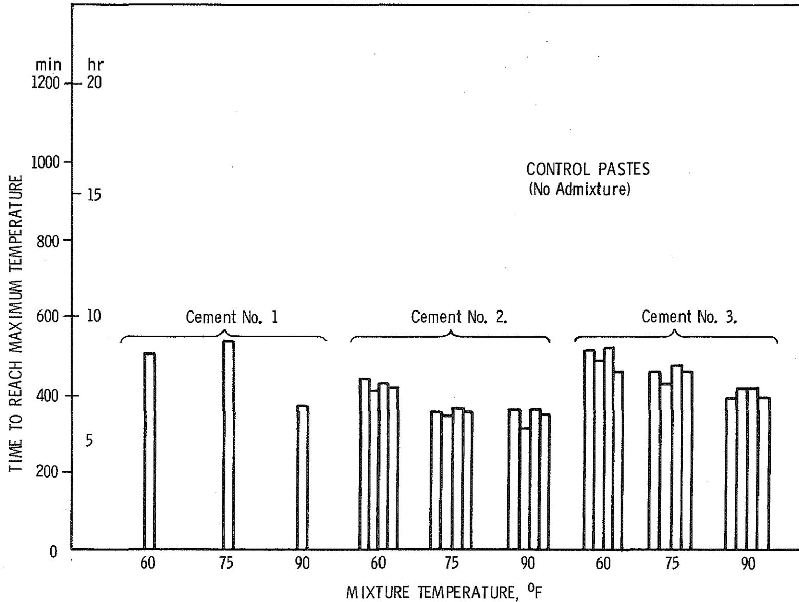
Figure 7. Time to reach maximum temperature for control pastes (no admixture). Four repeat tests at each mixing temperature for cements Nos. 2 and 3.
