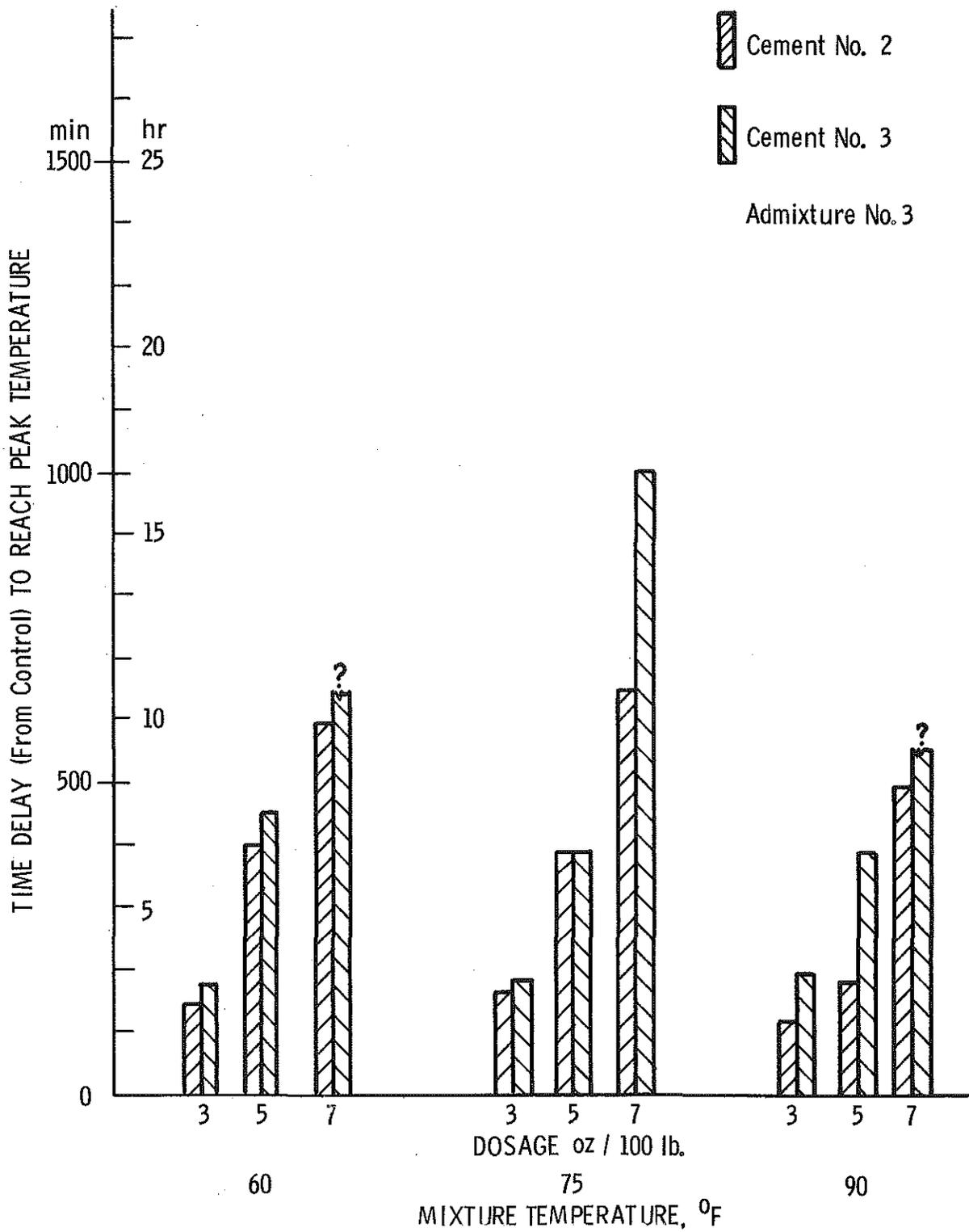
Figure 13. Delay from control in reaching peak temperature of pastes made with admixture No. 3.
