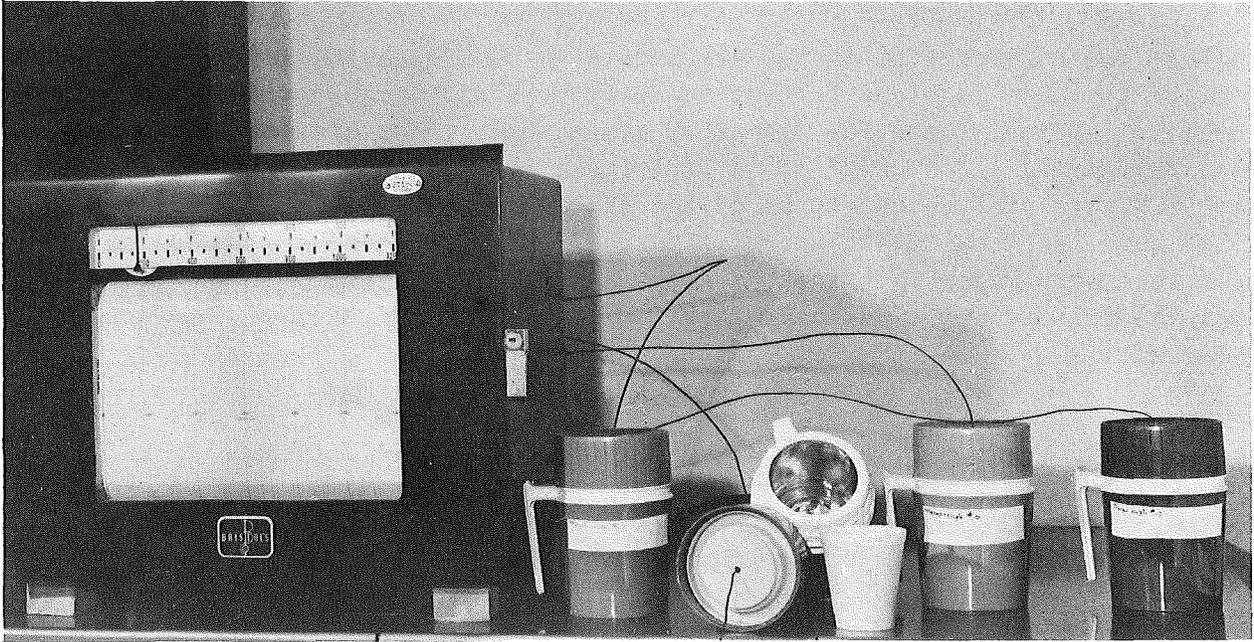
Figure 2. Automatic 10-point temperature recorder with four vacuum flasks, one opened to display paste cup, flask cover, and glass thermocouple protector.
