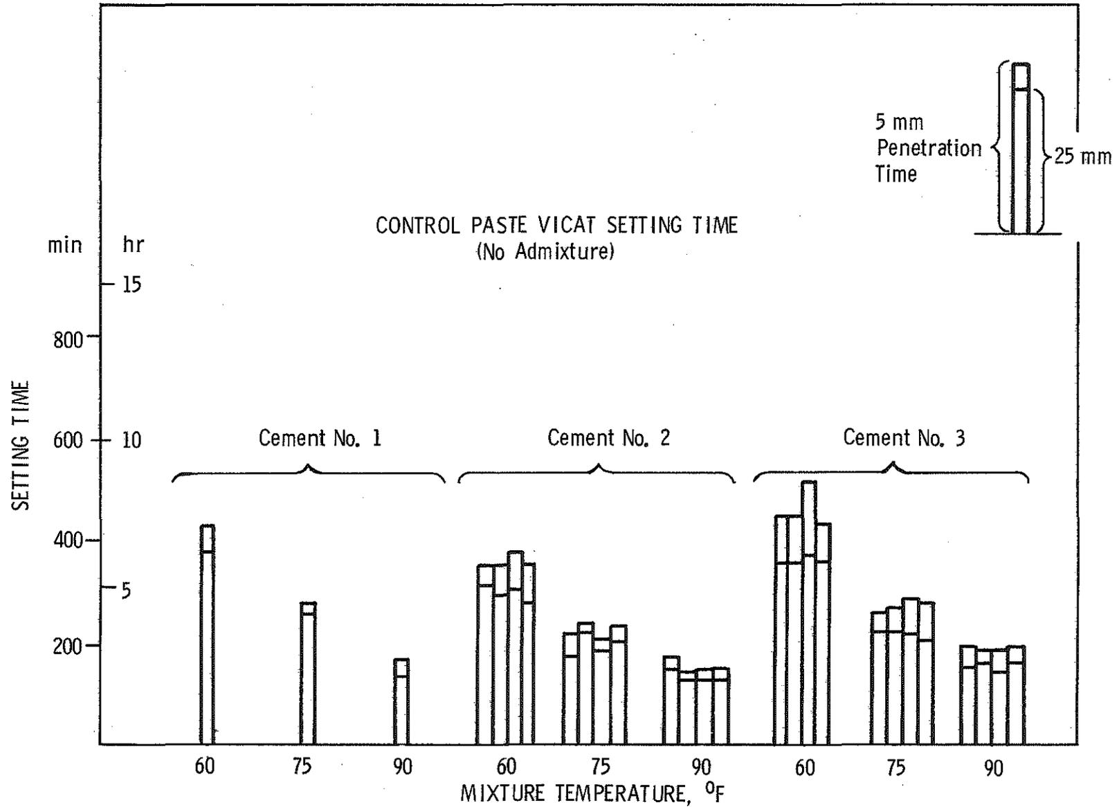
Figure 9. Control paste vicat setting time (no admixture). Four repeat tests for each mixing temperature for cements Nos. 2 and 3.
