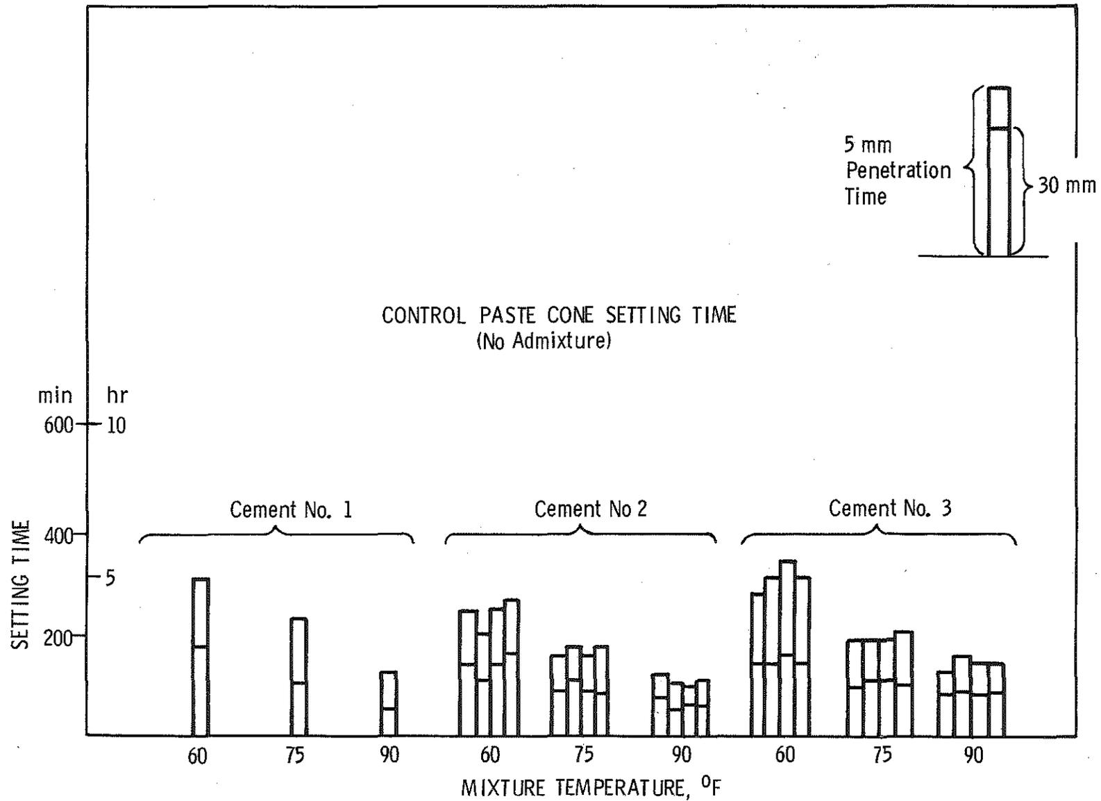
Figure 10. Control paste setting time using 20° blunted cone loaded to 250 g (no admixture). Four repeat tests for each mixing temperature for cements Nos. 2 and 3.
