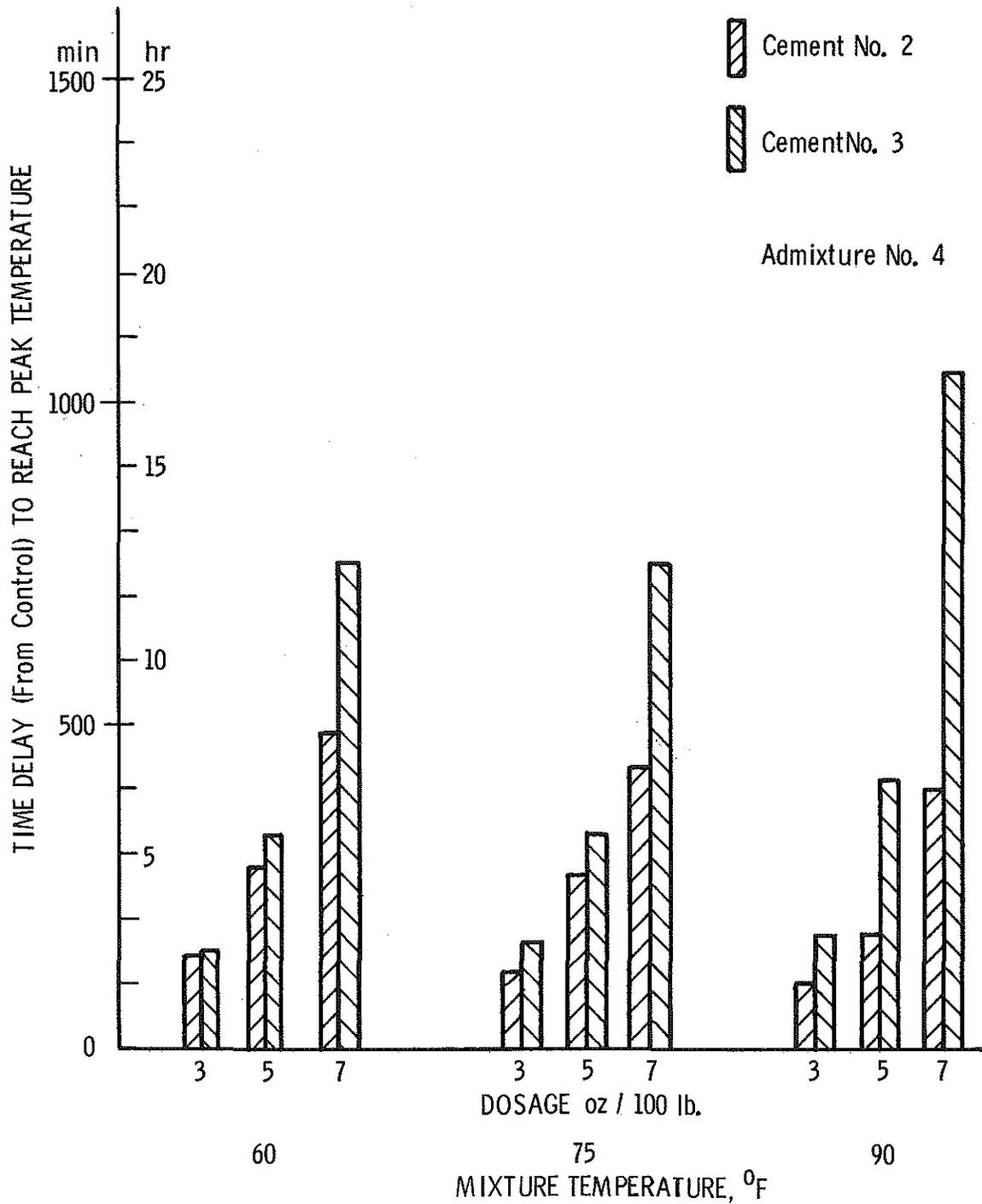
Figure 14. Delay from control in reaching peak temperature of pastes made with admixture No. 4.
