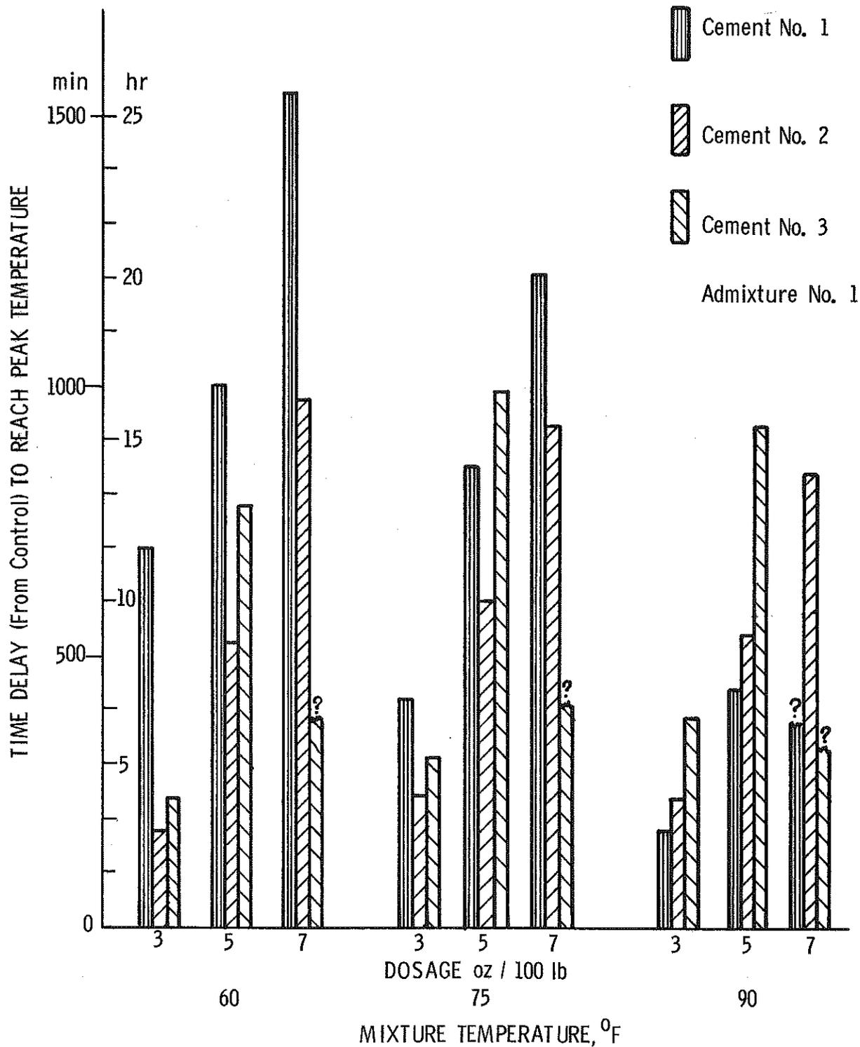
Figure 11. Delay from control in reaching peak temperatures of pastes made with admixture No. 1.
