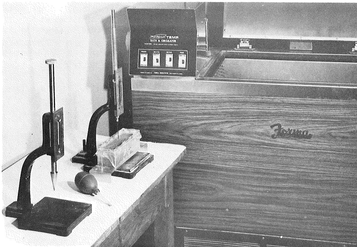
Figure 1. Vicat and cone cement paste penetrometers, paste setting time container, and constant temperature water bath.
