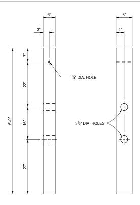
CONTROLLED RELEASING TERMINAL POST ( CRT )
