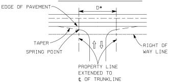
\*DRIVEWAYS INCLUDING RADII FOR EACH PROPERTY MUST BE LOCATED WITHIN THESE LIMITS UNLESS WRITTEN PERMISSION OF THE ADJACENT PROPERTY OWNER IS OBTAINED FOR PLACING A DRIVEWAY RADII OUTSIDE OF THESE LIMITS.
